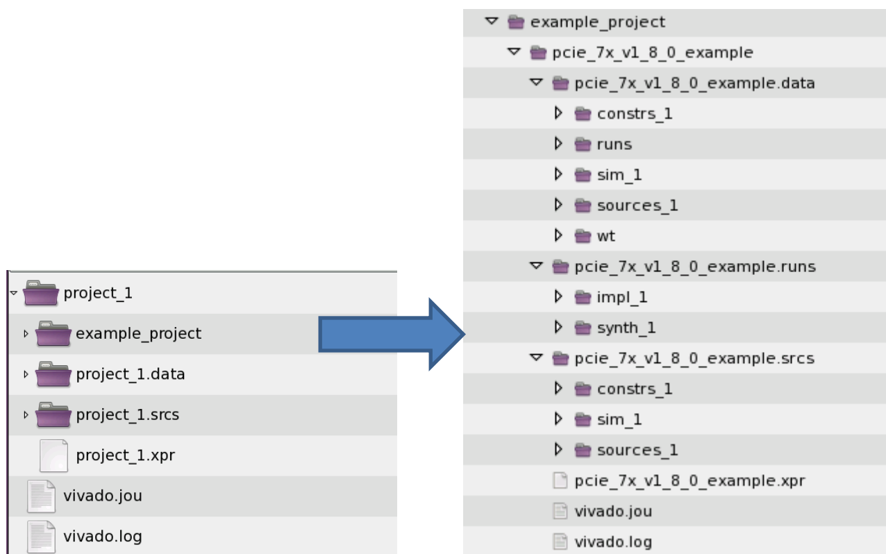
Figure 26 – 'example_project' content after PCIe Example Design Implementation
