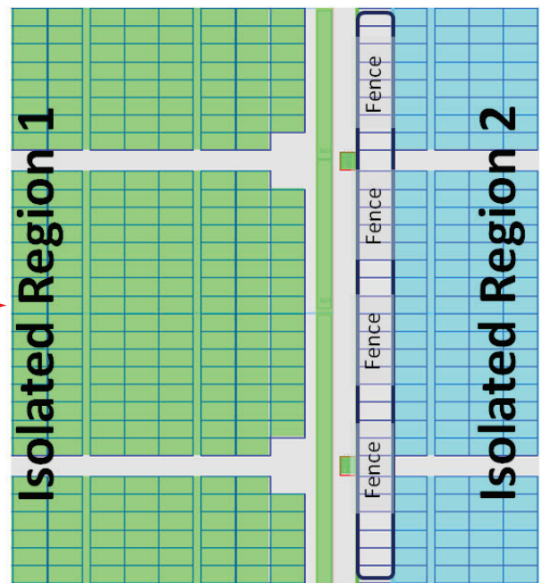
Figure 23: Invalid and Valid Fence Placement Adjacent to Clock Column (DCM/PLL)
