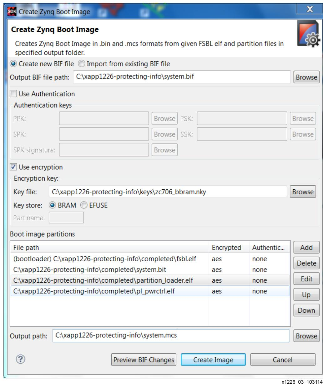
Figure 3: Bootgen BIF in GUI
