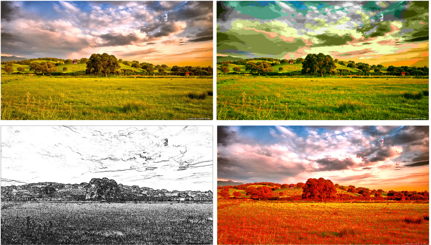
Figure 2: Comparing Image Filters: Original (top left), Posterize (top right), Sobel (bottom left), FAST (bottom right)
