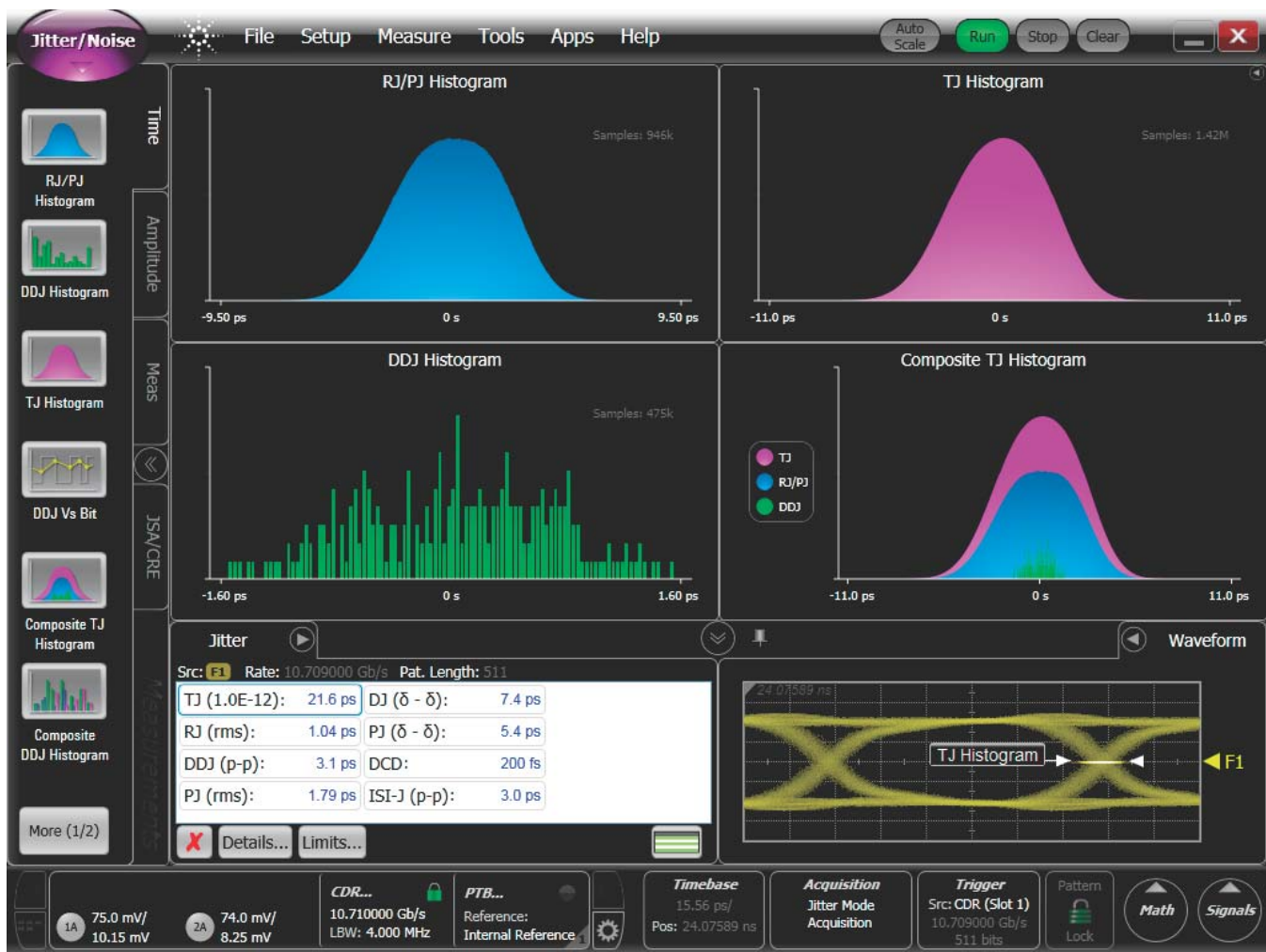
Figure 7: Output 10.71 Gb/s 100 ppm Offset
