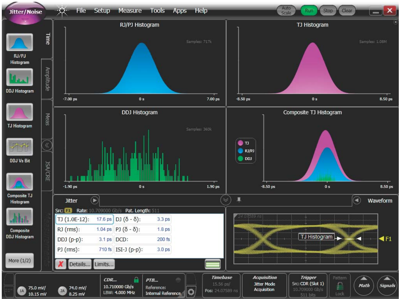
Figure 6: Output 10.71 Gb/s 20 ppm Offset
