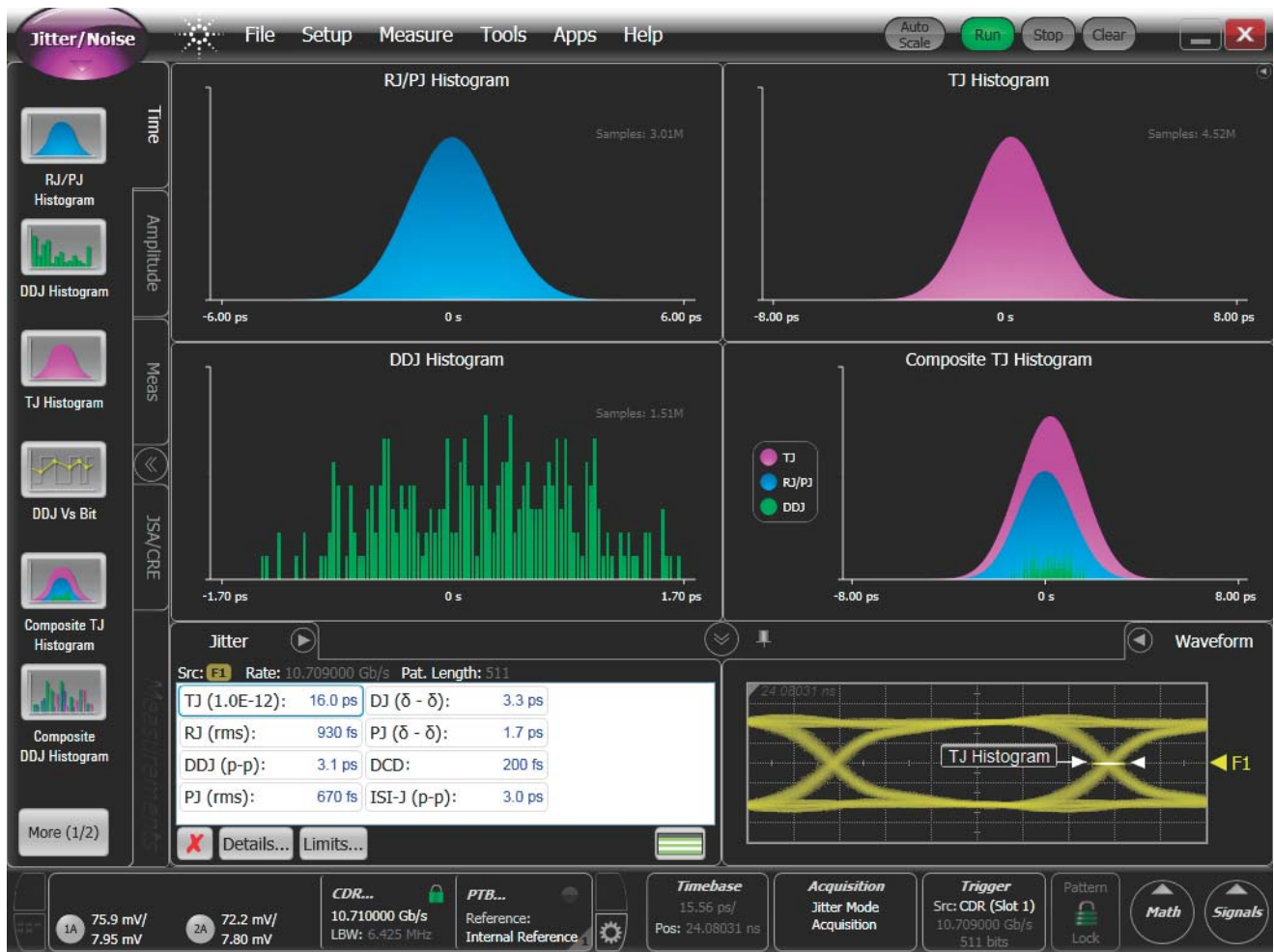
Figure 5: Output 10.71 Gb/s 0 ppm Offset
