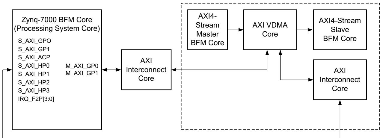
Figure 1: Reference System Block Diagram
