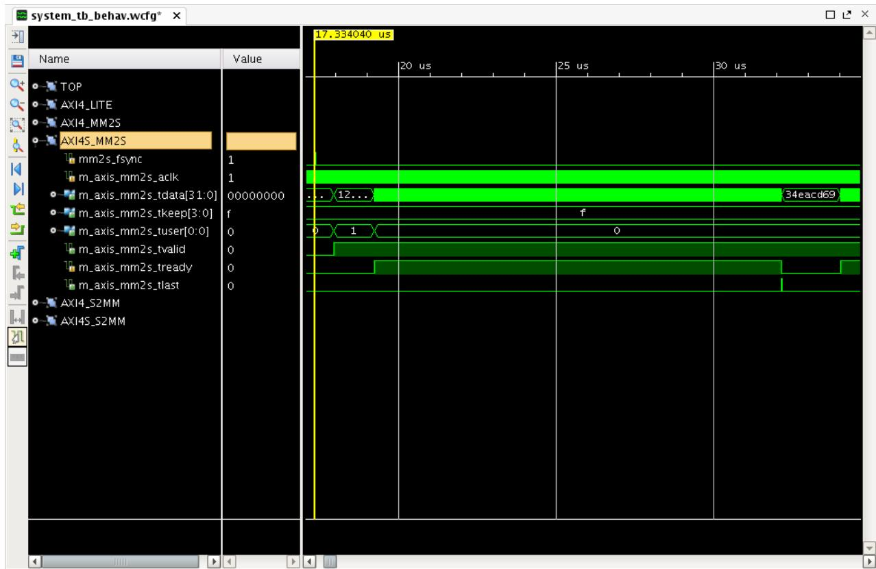
Figure 5: AXI4S\_MM2S–Horizontal Line Complete
