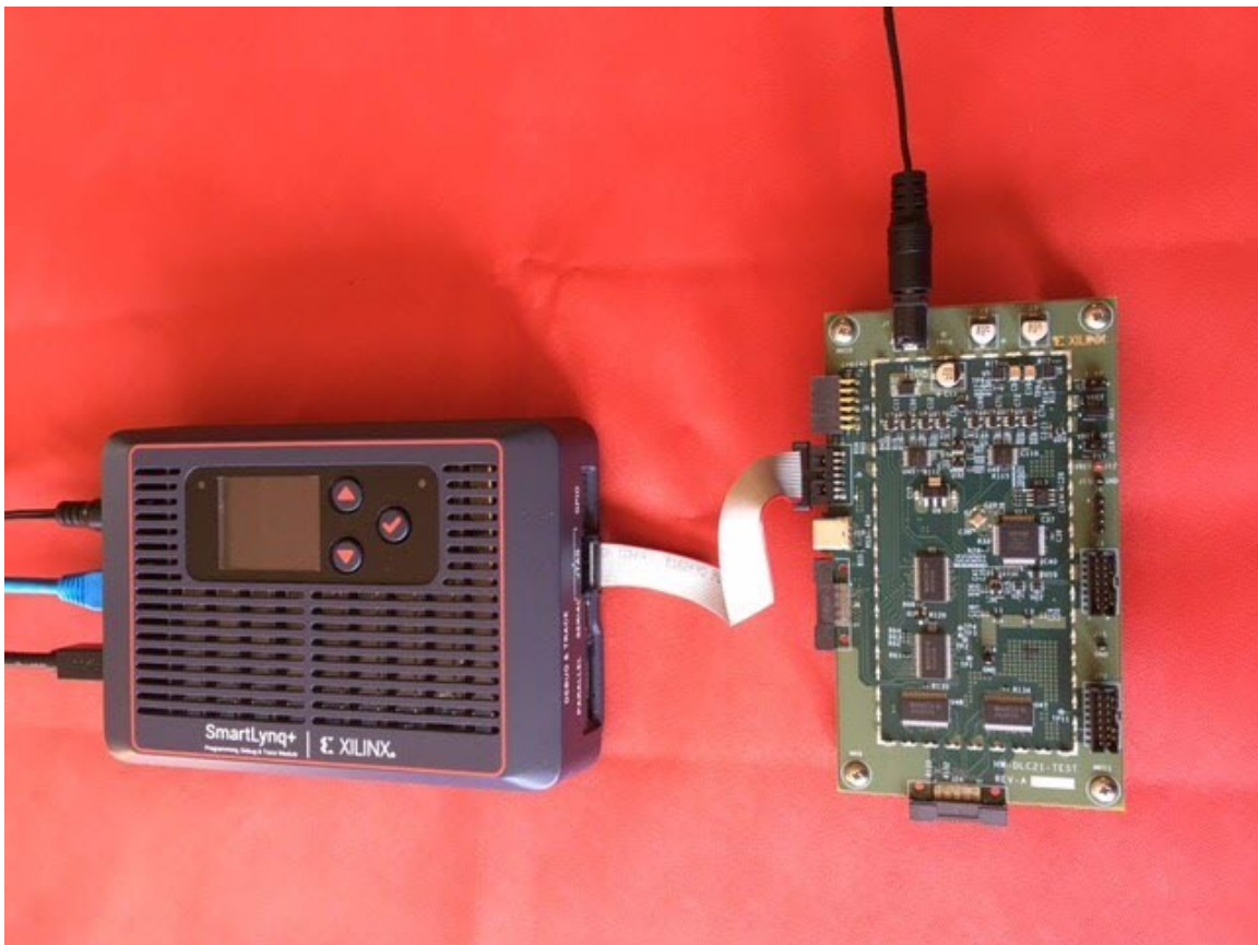
Figure 6: SmartLynq+Module JTAG Connection to the JTAG Interface on a Target Board
