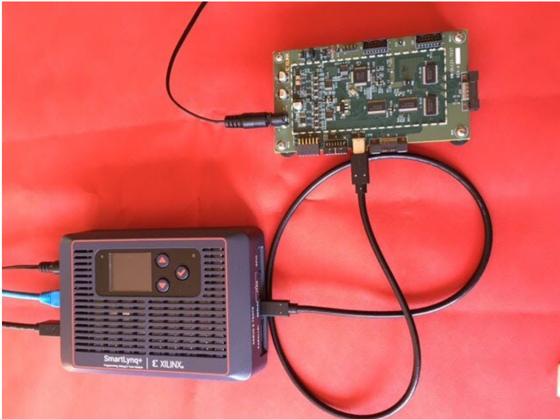
Figure 11: SmartLynq+ to HSDP on a Target Board
