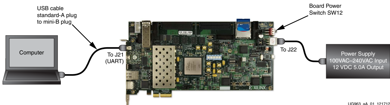
Figure A-1: Host Computer COM Port Configuration
