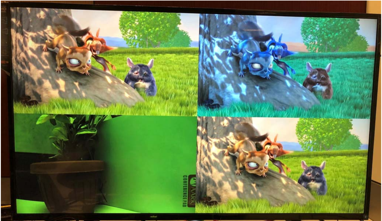
Figure 3-18: Multi-Stream—3 HDMI and 1 MIPI Input Sources @ 1080p60
