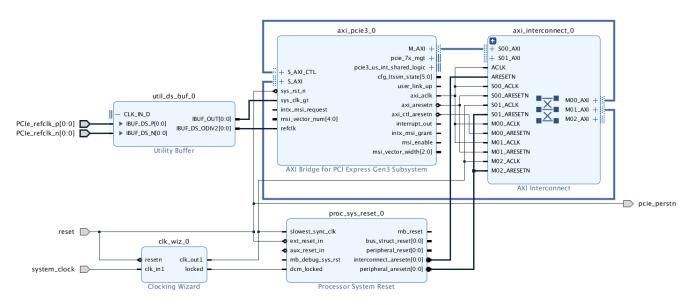
Figure 6: Root Port System Reset Connection (UltraScale Devices)
