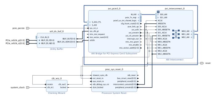
Figure 4: Endpoint System Reset Connection (UltraScale Devices)
