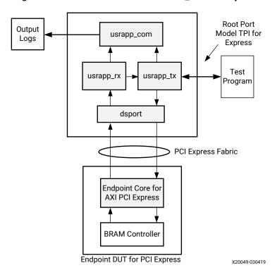
Figure 40: Root Port Model for AXI\_PCIE Endpoint
