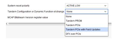
For complete information about Tandem Configuration, including required PCIe block locations, design flow examples, requirements, restrictions and other considerations, see Tandem Configuration in the UltraScale Devices Gen3 Integrated Block for PCI Express LogiCORE IP Product Guide (PG156). For information on Dynamic Function eXchange, see the Vivado Design Suite User Guide: Dynamic Function eXchange (UG909).
