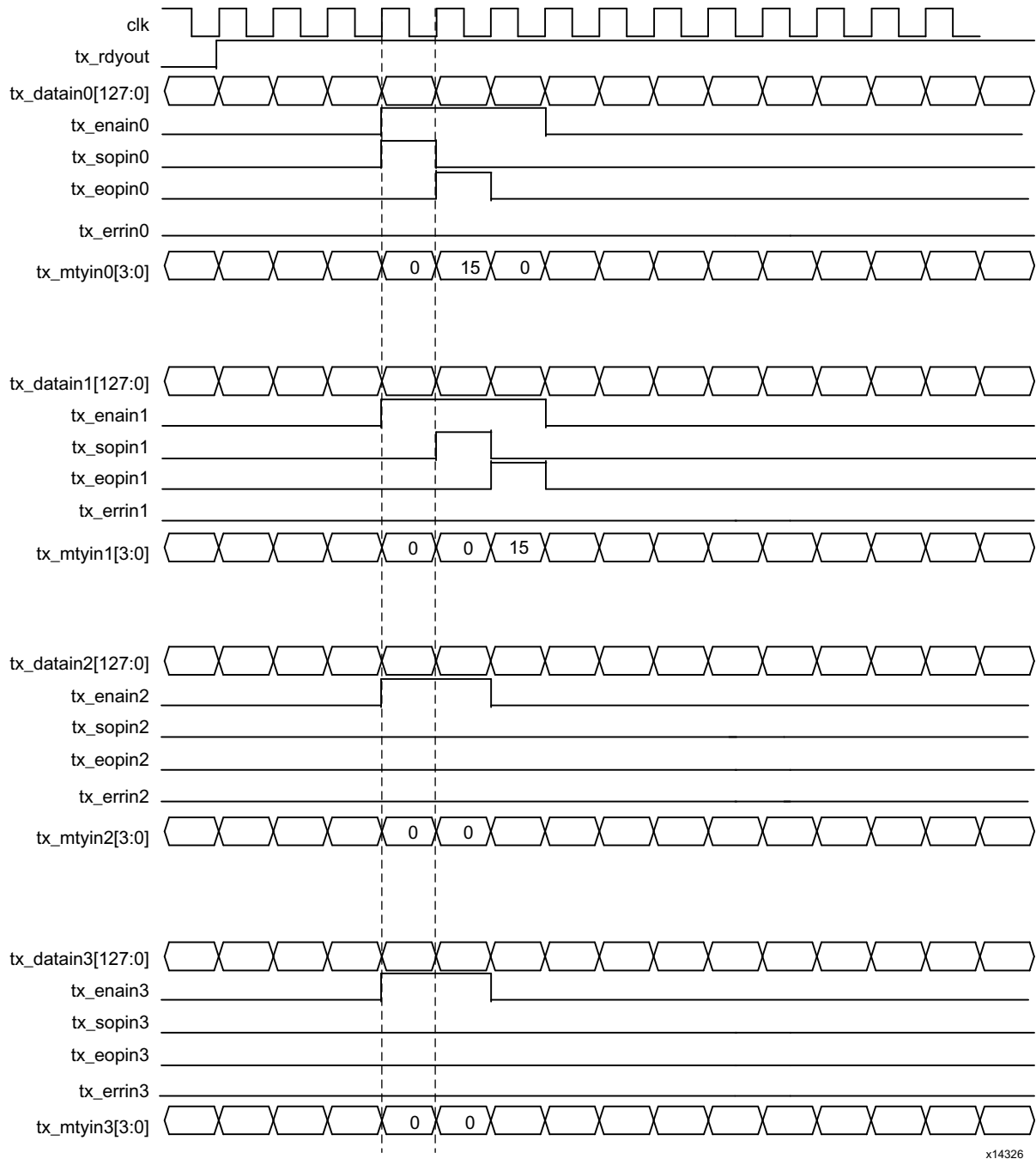
Figure 3-7: Transmit Timing Diagram
