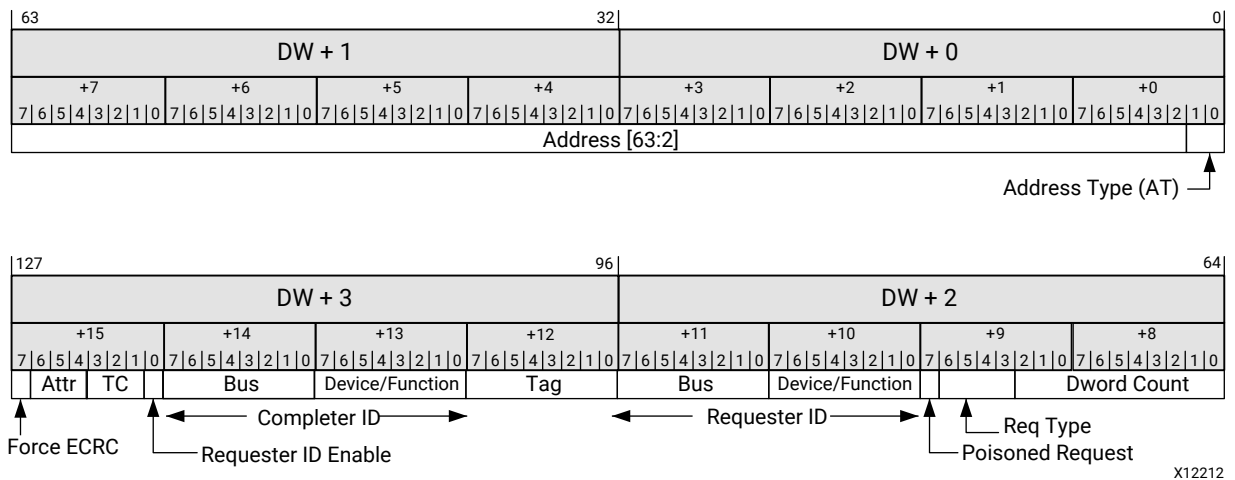
Figure 77: Requester Request Descriptor Format for Memory, I/O, and Atomic Op Requests
