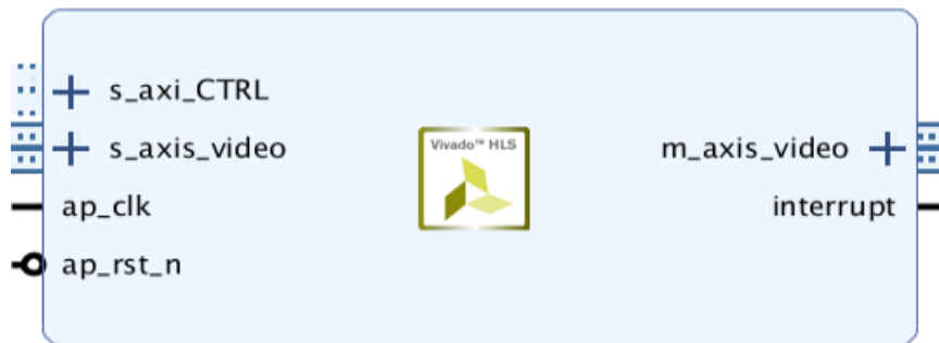
Figure 2: Scene Change Detection IP I/O Diagram Stream Mode
