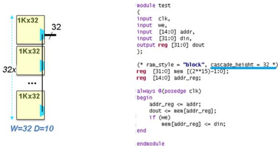
Figure 3-30: RTL Representation of 32Kx32 Using 1Kx32 and CASCADE_HEIGHT=32
