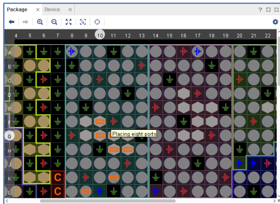
Figure 3-17: I/O Ports Placed in I/O Banks
