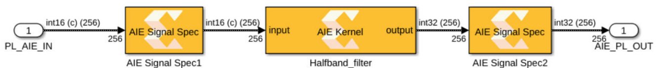
Figure 267: AIE Signal Spec Block Connected to AI Engine Subsystem
