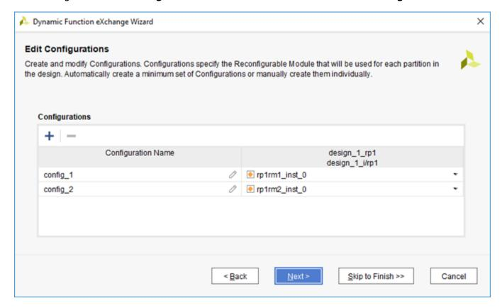
**Note:** If one RM is used in more than one Configuration, the implementation results may be different, as place and route is performed each time, but only if the RM was initially implemented in a child run. RM implementation results will be reused if they were originally done in the parent configuration. This allows the Vivado project to track dependencies between parent and child.
