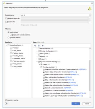
This set of DRCs can be run from the Tcl Console or within a script, by using the  $report_drc$  command. To limit the checks to the ones shown here for Partial Reconfiguration, use this syntax:
