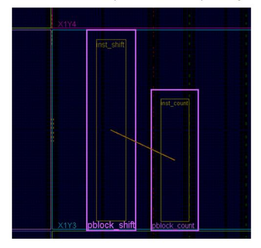
Figure 8: RESET\_AFTER\_RECONFIG Compatible (Left) and Incompatible (Right) Pblocks
