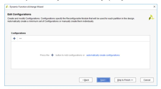
If one Partition Definition has more RMs than another, a graybox RM will automatically be used for any RP that has all its RMs covered by prior Configurations. These default Configurations can be modified or renamed, and additional Configurations may be created if desired.
