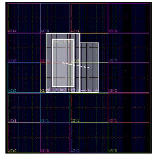
Figure 71: Supported Stair-Step Shaped Pblock
