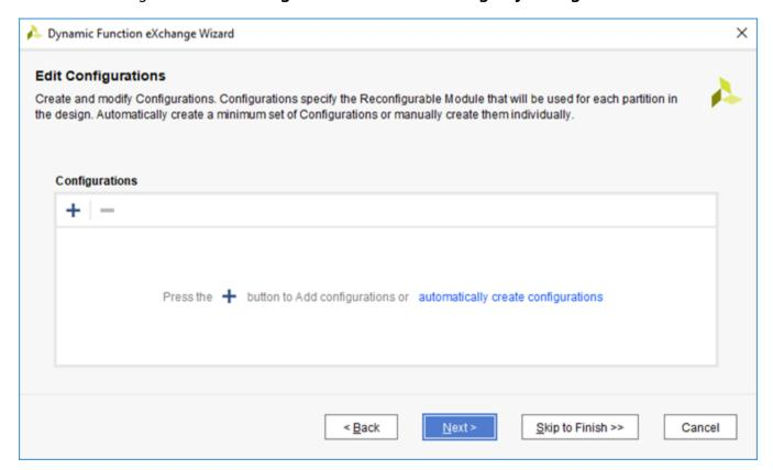
If one BDC has more RMs than another, a graybox RM will automatically be used for any RP that has all its RMs covered by prior Configurations. These default Configurations can be modified or renamed, and additional Configurations may be created if desired.
