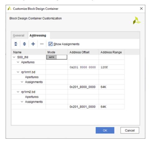
Figure 48: Viewing the Address Aperture for a BDC
