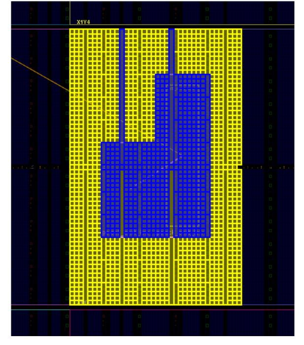
Figure 67: Highlighted Pblock and Expanded Routing Footprint
