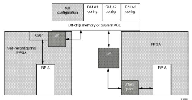
Figure 113: Configuring Through a Microprocessor
