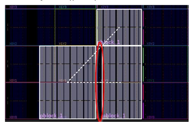
Figure 73: Unsupported Gap in the IOB Column
