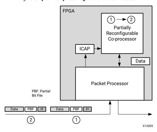
Figure 5: Dynamically Reconfigurable Packet Processor
