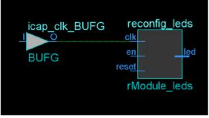
If there are a large number of global clocks driving an RP, create area groups that encompass complete clock regions to ease placement and routing of static logic. Global clocks can be downgraded to regional clocks (for example, BUFR, BUFH) for clocks with fewer loads or less demanding requirements. Shifting clocks from global to local resources allows for more flexibility in floorplanning when the RP requires many unique clocks.
