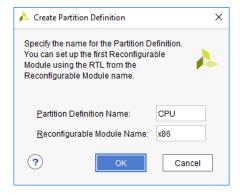
3. After clicking **OK**, this module displays differently in the Vivado IDE. Each instance of the module is shown in the Hierarchy view with a diamond, indicating that it is a RP. The design sources are moved to the Partition Definitions view to be managed separately. Repeat this step for all unique RPs required within the design.
