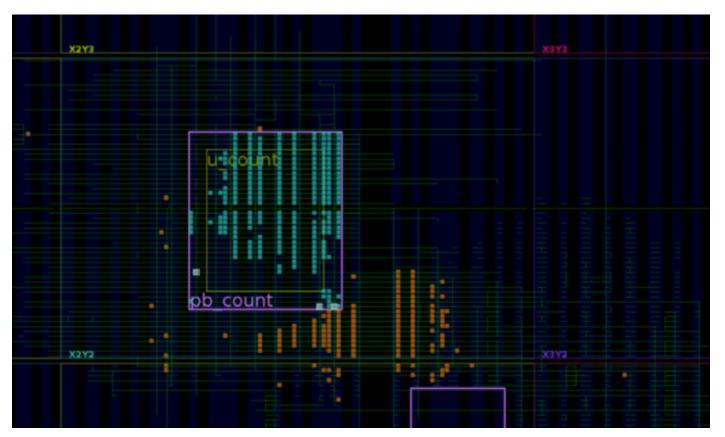
Figure 18: Routed Reconfigurable Module within an Abstract Shell
