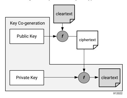
Figure 6: Asymmetric Key Encryption
