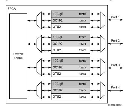
Figure 2: Network Switch Without Partial Reconfiguration
