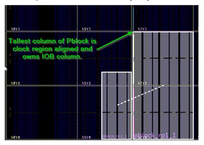
Figure 72: Tallest Column of Pblock Clock Region Aligned
