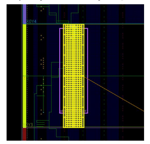
Figure 59: Original and Derived Pblocks Using SNAPPING\_MODE
