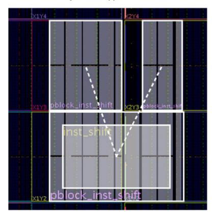
Figure 70: Supported Pblock with Small Static Gap
