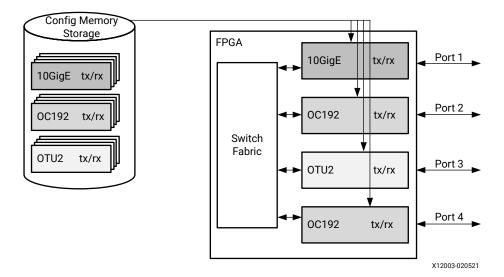
Figure 3: Network Switch With Partial Reconfiguration
