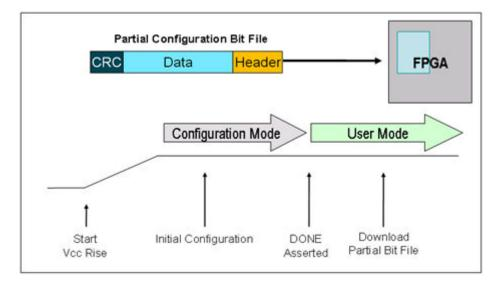
Figure 112: Configuring with a Partial BIT File
