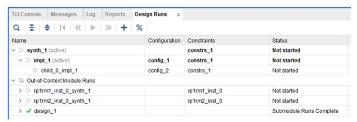
In the **Design Runs** window, out-of-context synthesis runs are created for each RM, and all **Configuration Runs** are generated. Relationships between parent and child runs are shown by the levels of indentation.
