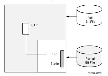
Figure 4: Configuration by Means of PCIe Interface
