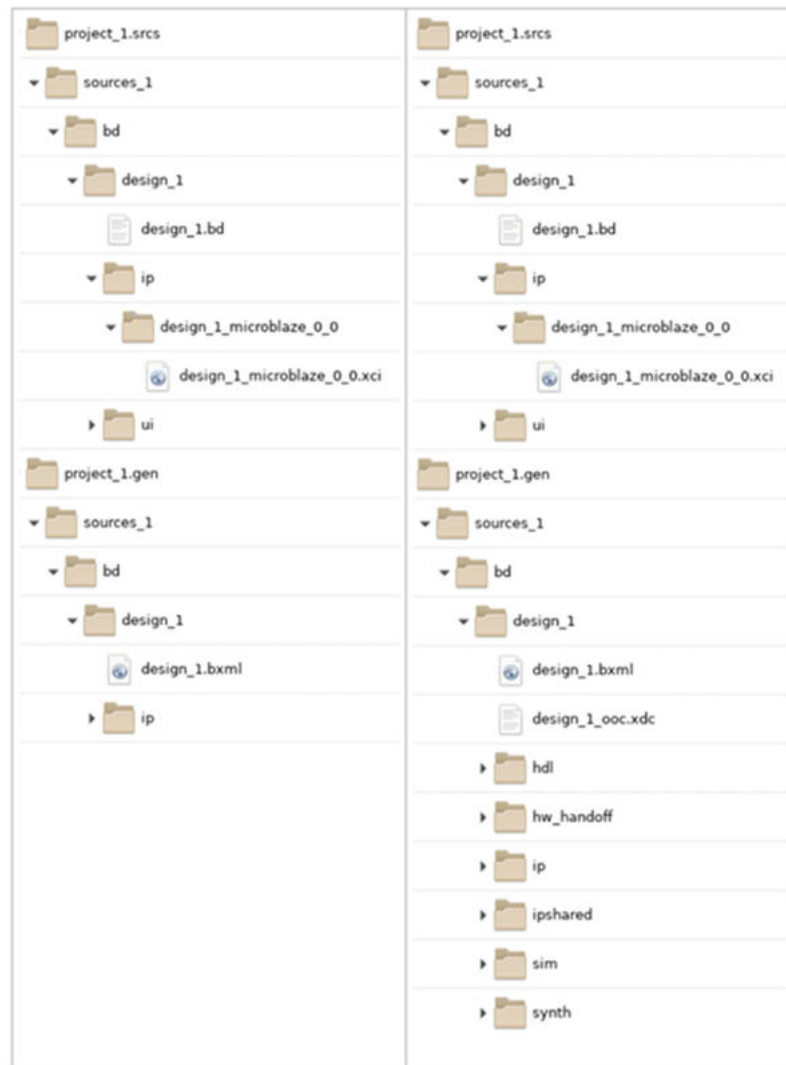
Figure 138: Directory Structure for Project IP and BD Files Before (Left) and After (Right) Generate Design
