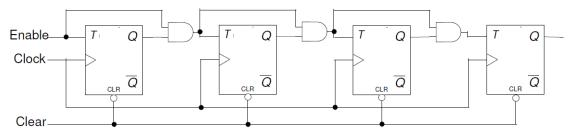
2-1. Design a 8-bit counter using T flip-flops, extending the above structure to 8-bits. Your design needs to be hierarchical, using a T flip-flop in behavioral modeling, and rest either in dataflow or gate-level modeling. Develop a testbench and validate the design. Assign Clock input to SW0, Clear\_n to SW1, Enable to SW2, and Q to LED7-LED0. Implement the design and verify the functionality in hardware.
