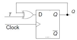
2-2. Modify the 8-bit counter using D flip-flops. The design should be hierarchical, defining D flip-flop in behavioral modeling, creating T flip-flop from the D flip-flop, implementing additional functionality using dataflow modeling. Assign Clock input to SW0, Clear\_n to SW1, Enable to SW2, and Q to LED7-LED0. Implement the design and verify the functionality in hardware.
