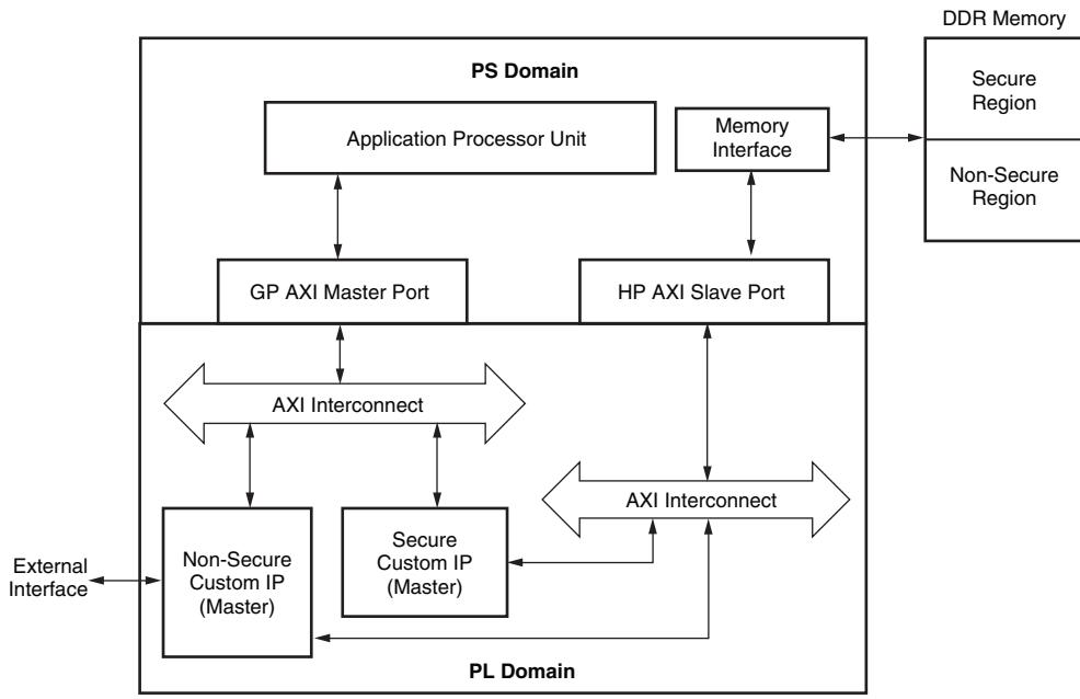
**Figure 4: Conceptual System using Zynq-7000 AP Soc Technology**
