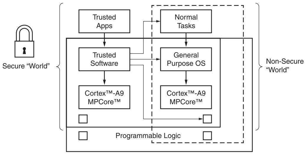
**Figure 1: Trusted and Non-Trusted Applications on a Zynq-7000 AP SoC**
