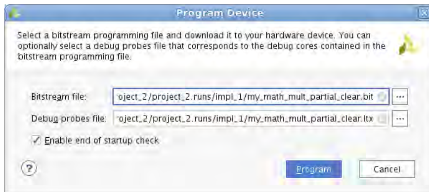
Figure 77: Selecting the clearing bitstream that corresponds to the current RM
