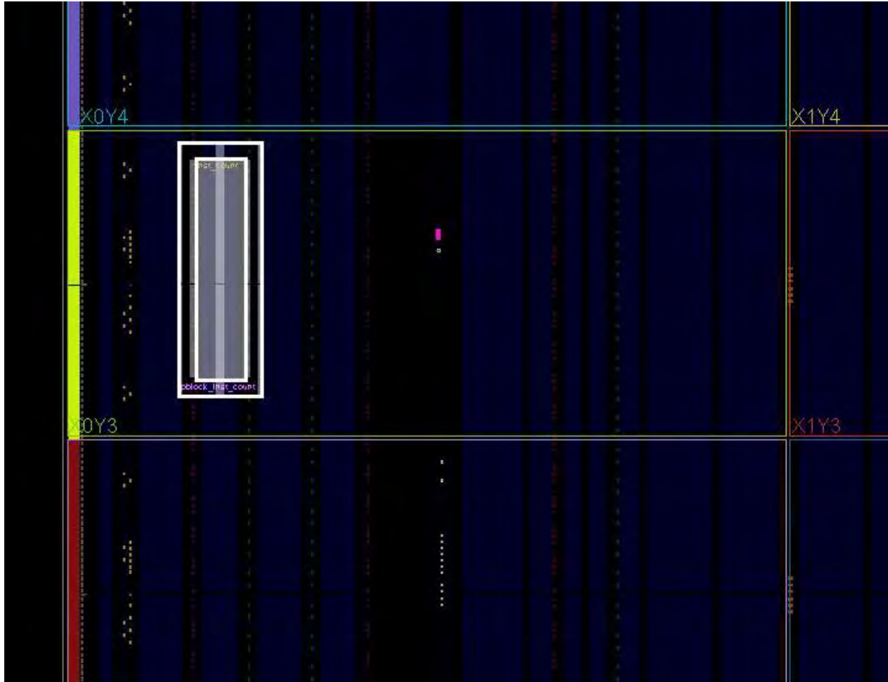
Figure 1: Pblock for the inst_count Reconfigurable Partition
