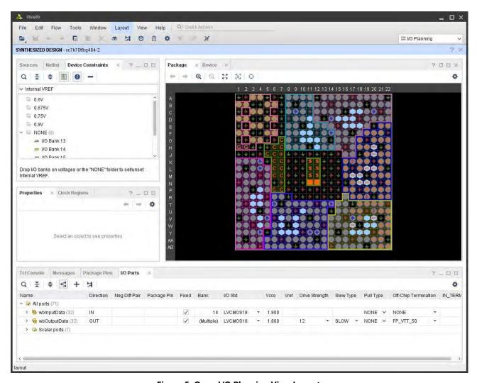
Figure 5: Open I/O Planning View Layout
