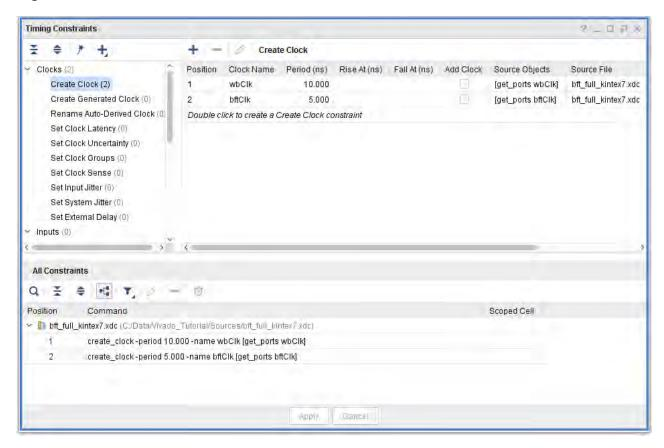
**Figure 3: Define Timing Constraints**
