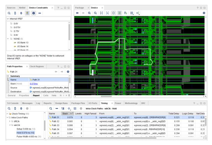
**Figure 30: Examine Routing for Timing Paths**
