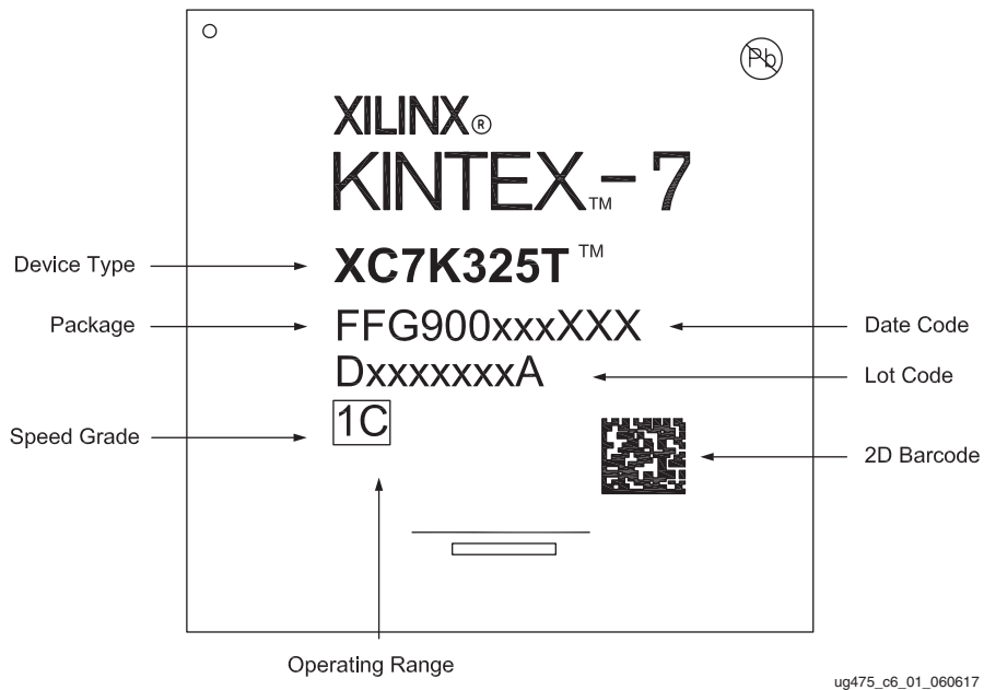
Figure 6-7: Legacy Kintex-7 Device Package Marking
