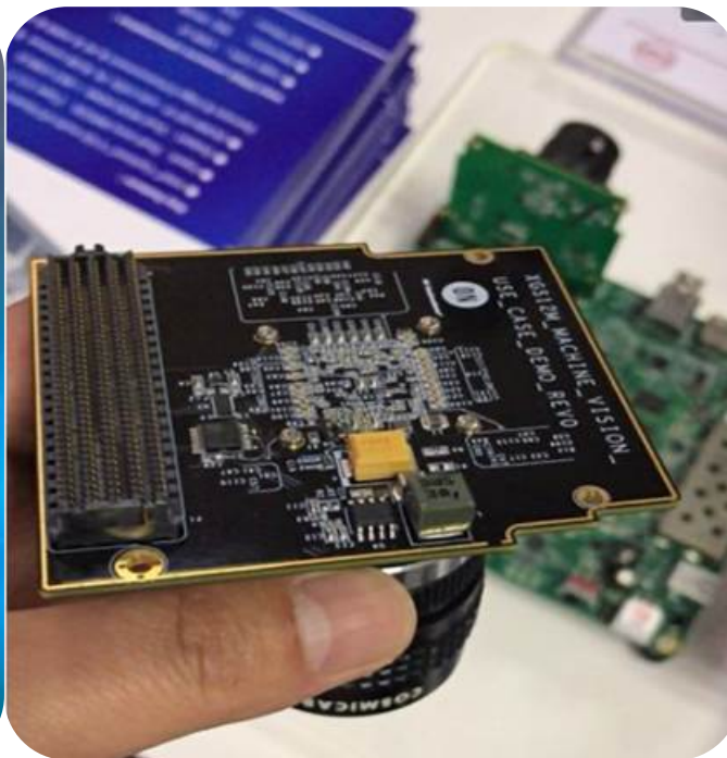
ZCU104 Demo for HiSPi XGS 12000 – 4K CMOS Global Shutter
