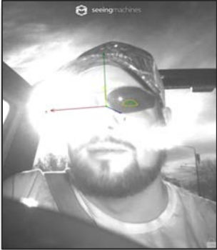
Typical driving situation Driver wearing sunglasses in full sun 1.3MP NIR sensor.
