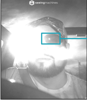
Algorithms control contrast in eye image region by selecting optimal intensity and energy of NIR pulse matched to imager control settings.
