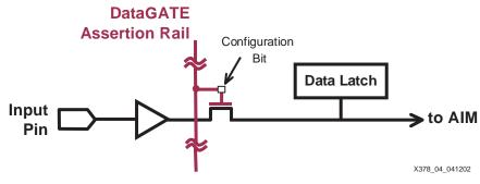
Figure 4: DataGATE Block Diagram
