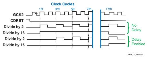
Figure 2: Clock Divider Waveform
