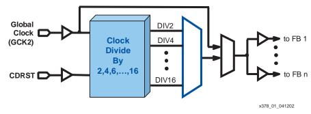
Figure 1: CoolRunner-II Clock Divider
