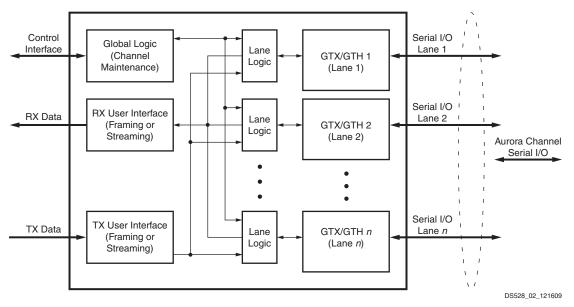
Figure 2: Aurora 64B/66B Core Block Diagram
