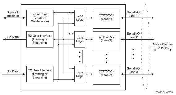
Figure 2: Aurora 8B/10B Core Block Diagram
