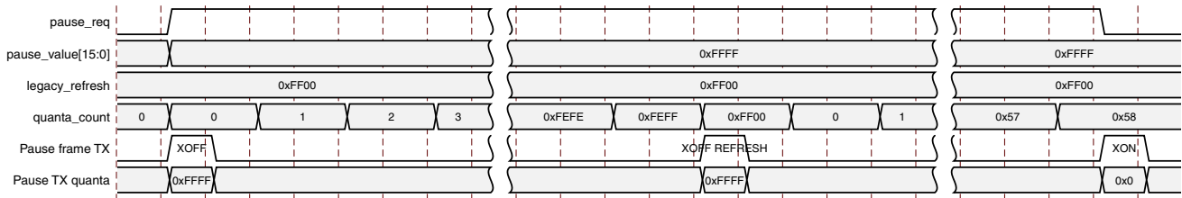
Figure 3-33: XON/XOFF Frame Transmission
