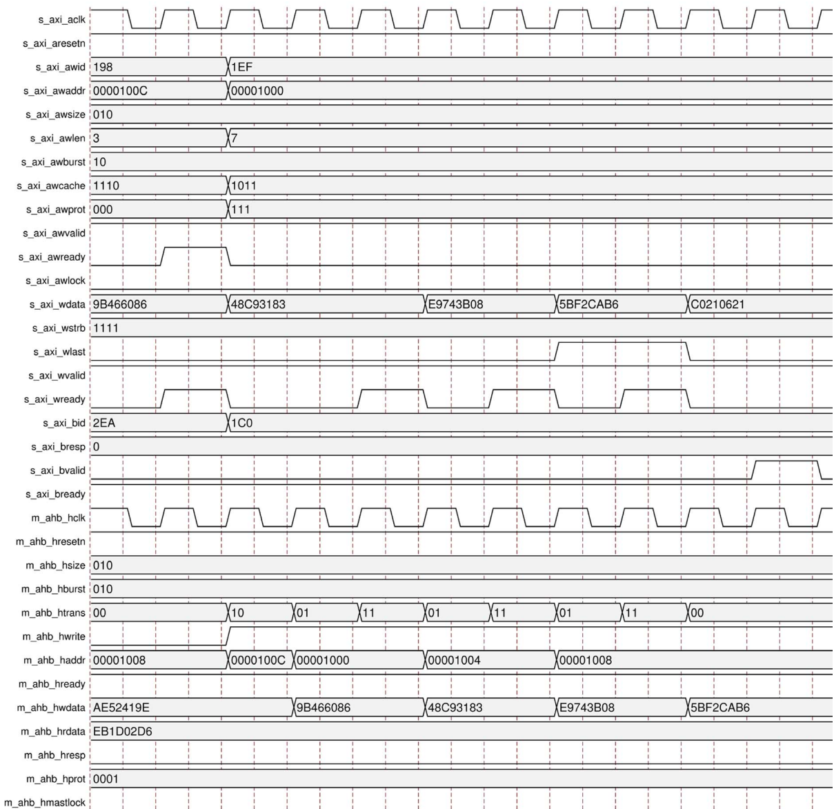
Figure 3-9: AXI4 Wrapping Burst Write Transfer of Length 4
