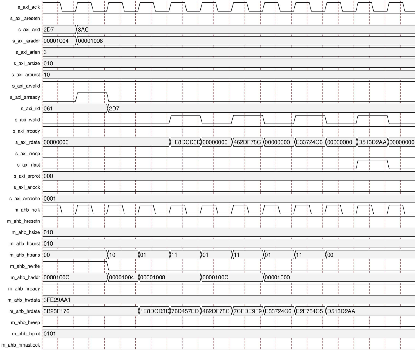
Figure 3-8: AXI4 Wrapping Burst Read Transfer of Length 4
