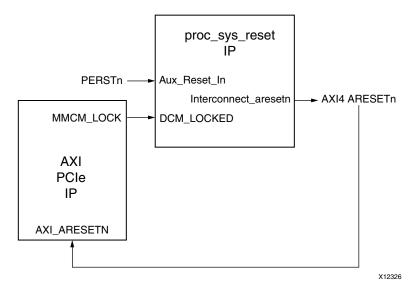
Figure 3-2: System Reset Connection
