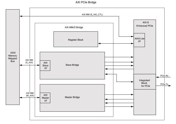
The architecture of the AXI Bridge for PCI Express is shown in Figure 1-1.
