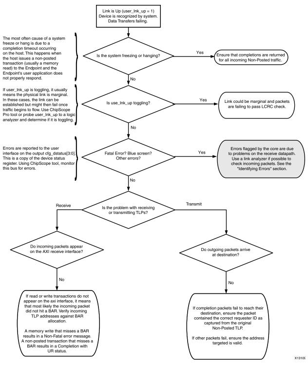
Figure B-6: Data Transfer Debug Flow Diagram
