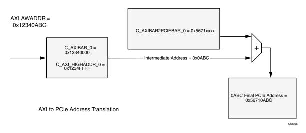
Figure 3-3: AXI to PCIe Address Translation
