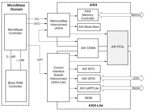
Figure 2-2: FPGA System Configuration Diagram
