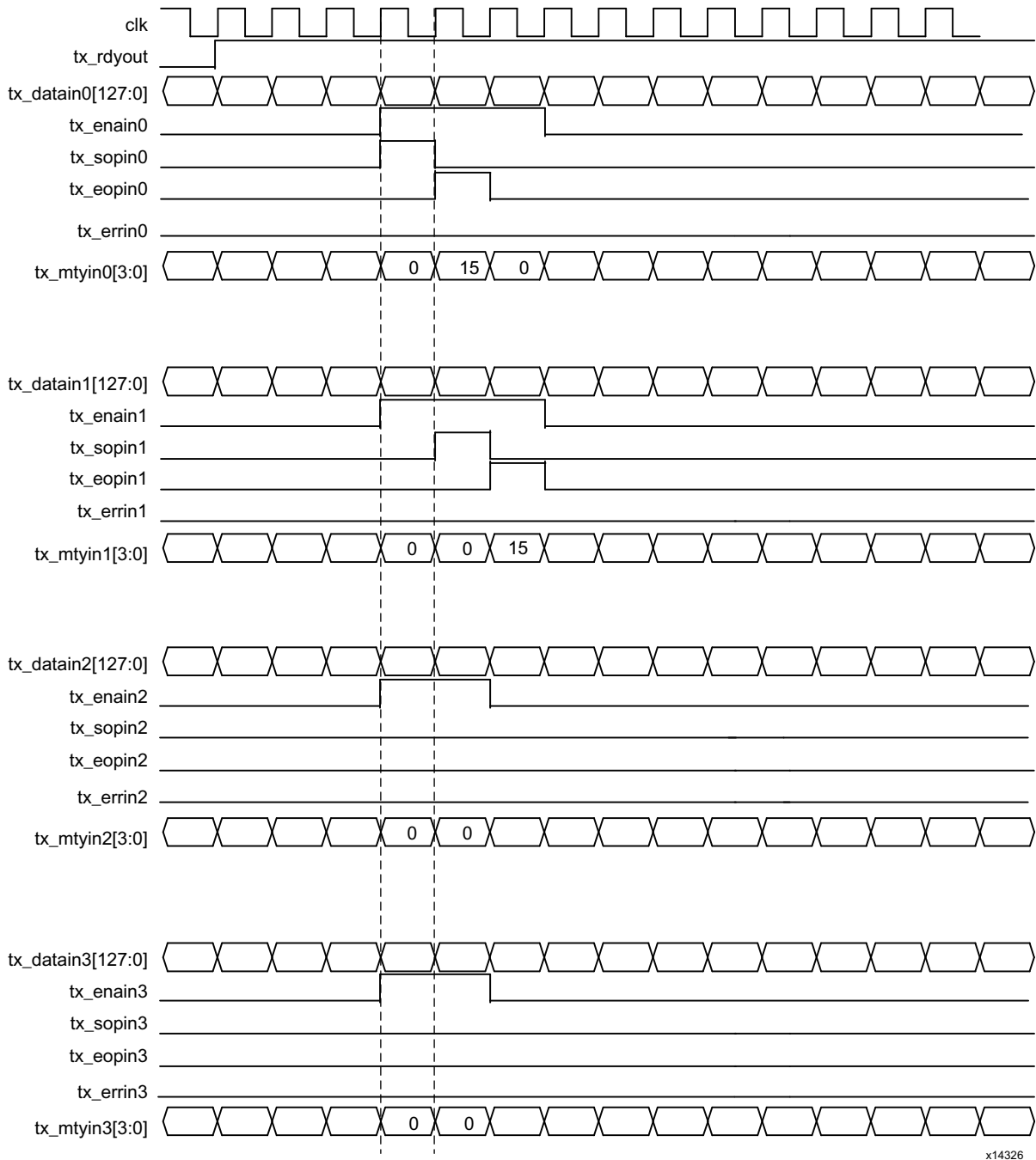
Figure 3-9: Transmit Timing Diagram
