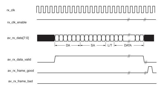
Figure 7: Normal Frame Reception across the AV Traffic Interface
