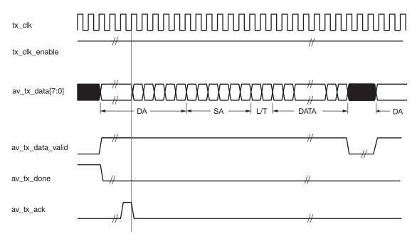
Figure 6: Normal Frame Transmission across the AV Traffic Interface
