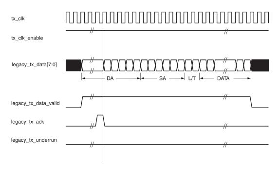
Figure 4: Normal Frame Transmission across the Legacy Traffic Interface
