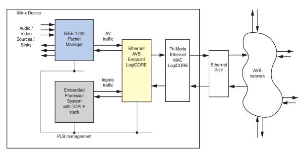
Figure 2: Example Ethernet AVB Endpoint System
