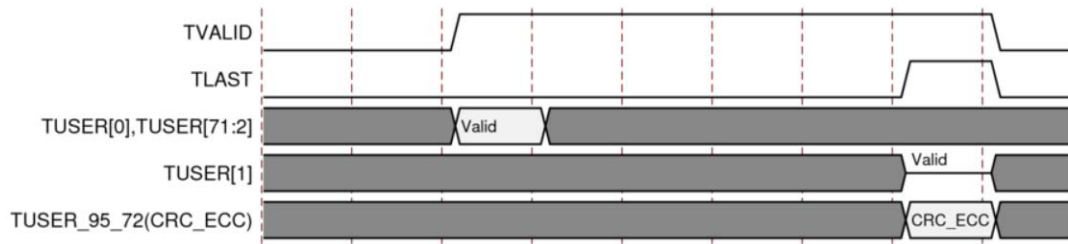
Figure B-1: Sideband Information (TUSER) Timing Diagram
