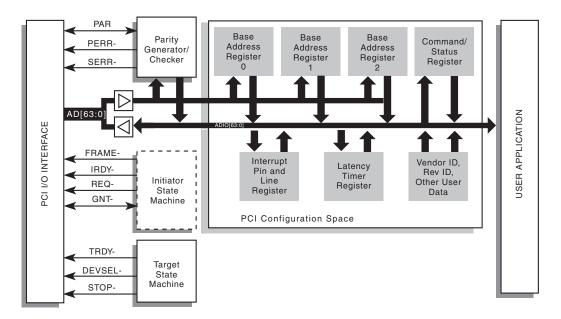
Figure 1: Initiator/Target Core for PCI Block Diagram
