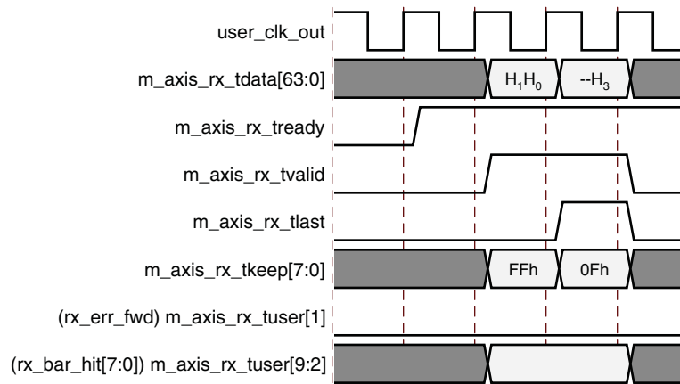
Figure 3-15: TLP 3-DW Header without Payload
