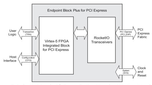
Figure 1: Endpoint Block Plus for PCI Express Top-Level Functional Blocks and Interfaces
