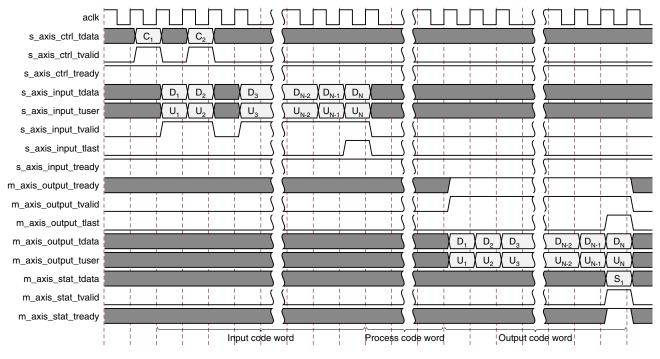
Figure 8: Block Input to Output Timing
