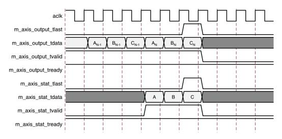
Figure 10: TLAST Timing for 3 Channel Example
