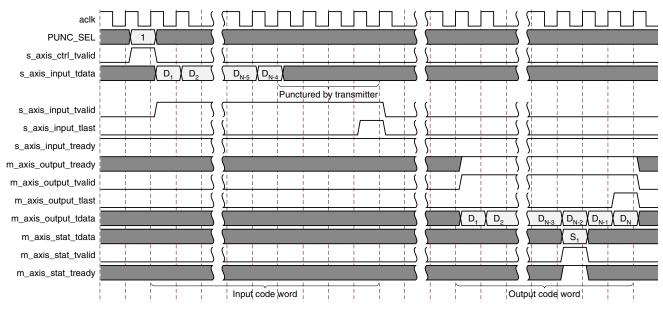
Figure 15: Puncture Timing
