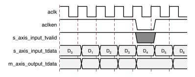
Figure 3: Clock Enable Timing
