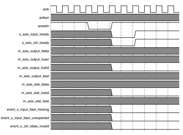
Figure 4: Synchronous Reset Timing
