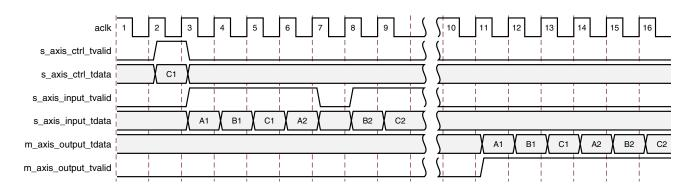
Figure 18: Multi-Channel Operation
