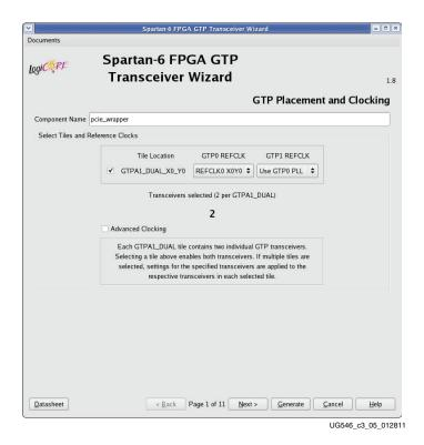
Figure 3-7: GTP Placement and Clocking—Page 1
