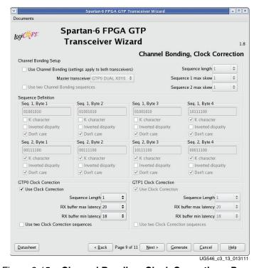
Figure 3-15: Channel Bonding, Clock Correction—Page 9
