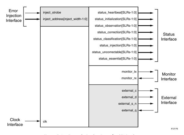
Figure 6-4: Example Design Ports for SSI Devices
