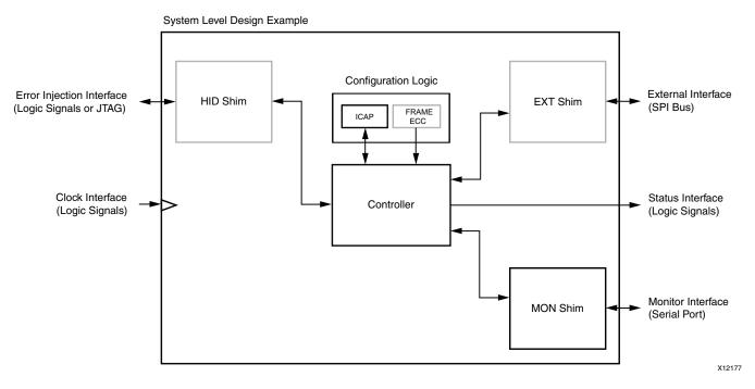
Figure 6-1: Example Design Block Diagram
