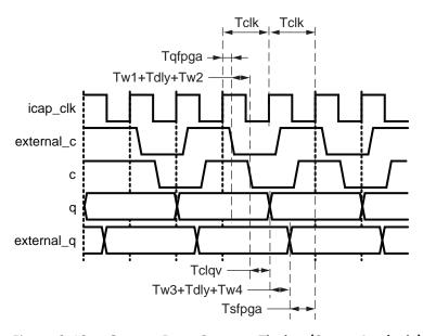
Figure 3-12: Output Data Capture Timing (Setup Analysis)
