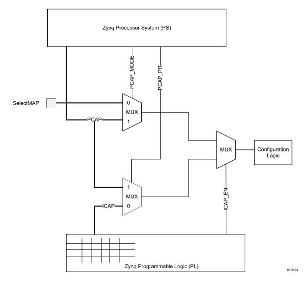
Figure 3-14: Configuration Logic Access in Zynq-7000
