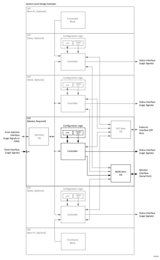
Figure 6-2: Example Design Block Diagram for SSI Devices
