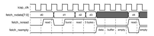
Figure 3-23: Fetch Interface Receive Protocol
