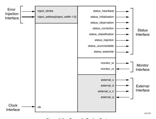
Figure 6-3: Example Design Ports
