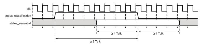
Figure 3-3: Status Interface Essential Flag Switching Characteristics
