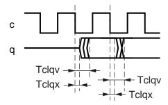
Figure 3-10: SPI Flash Device Output Data Switching Characteristics
