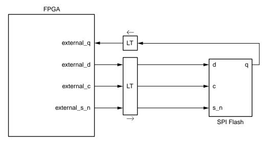
Figure 3-6: SPI Flash Device Connection, Including Level Translators
