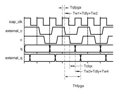
Figure 3-11: Output Data Capture Timing (Hold Analysis)
