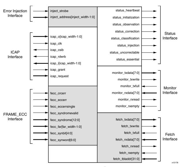
Figure 2-1: SEM Controller Ports
