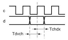
Figure 3-8: SPI Flash Device Input Data Capture Requirements
