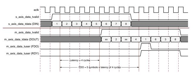
Figure 2-8: Forney Convolutional Interleaver Interface Timing
