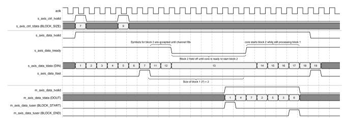
Figure 2-13: Loading Rectangular Blocks Back to Back
