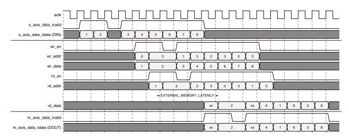
*Figure 3-10:* External RAM Interface Timing when EXTERNAL\_MEMORY\_LATENCY = 3
