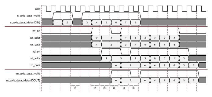
Figure 3-9: External RAM Interface Timing when EXTERNAL\_MEMORY\_LATENCY = 0
