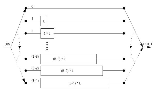
Figure 2-1: Forney Convolutional Interleaver
