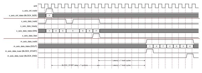
Figure 2-12: Rectangular Block Interface Timing
