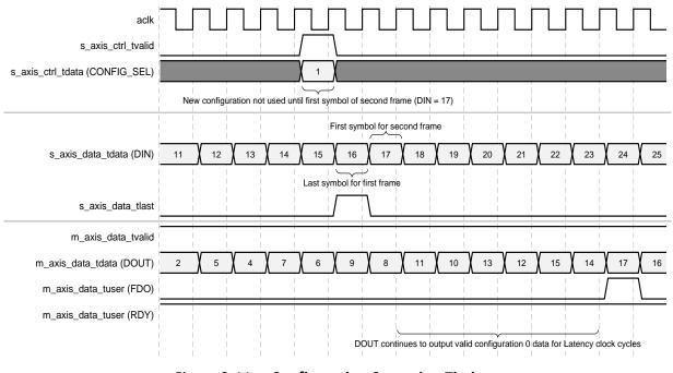
Figure 2-11: Configuration Swapping Timing
