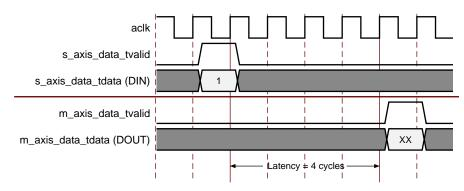
*Figure 2-9:* Forney Convolutional Interleaver Interface Timing - Wait states do not Affect Latency
