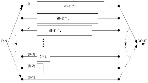
Figure 2-2: Forney Convolutional De-interleaver
