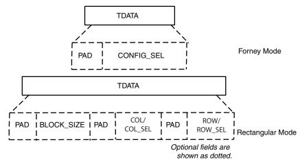
*Figure 3-5:* **Control Channel TDATA (s\_axis\_ctrl\_tdata) Format**
