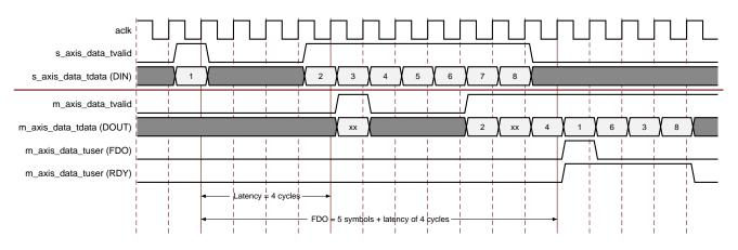
Figure 2-10: Forney Convolutional Interleaver Interface Timing - Wait states do Affect Delay
