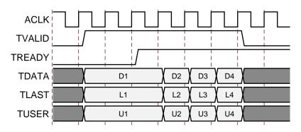
*Figure 3-1:* Data Transfer in an AXI4-Stream Channel
