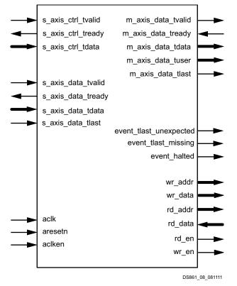
Figure 2-16: Forney Convolutional Schematic Symbol
