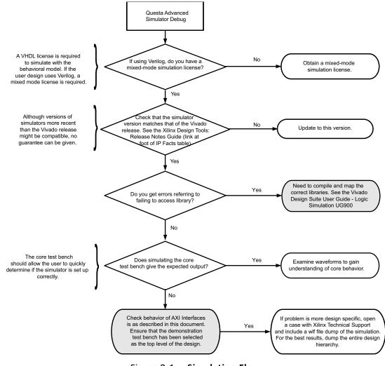
Figure B-1: Simulation Flow
