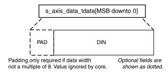
*Figure 3-2:* Data Input Channel TDATA (s\_axis\_data\_tdata) Format
