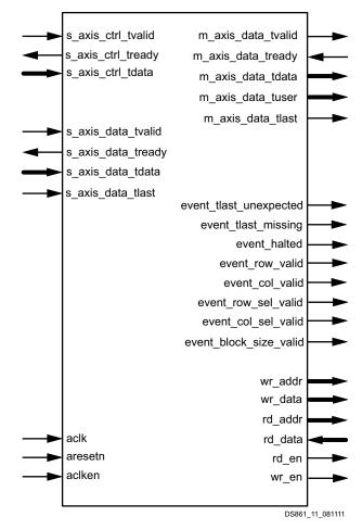
Figure 2-17: Rectangular Block Schematic Symbol
