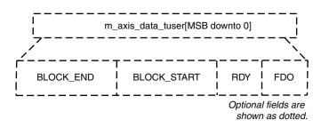
Figure 3-4: Data Output Channel TUSER (m\_axis\_data\_tuser) Format
