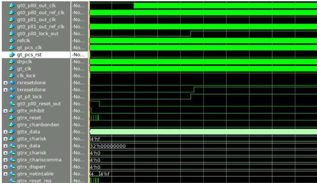
Figure C-6: GT Interface Signals
