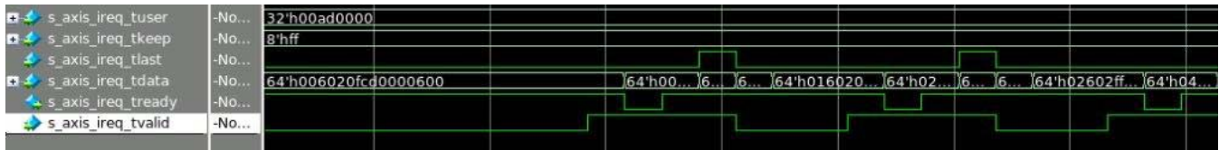
Figure C-7: SWRITE Packet Transmission on IREQ Interface
