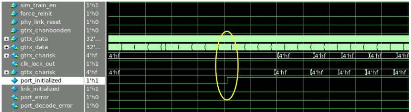
Figure C-3: port_initialized and link_initialized Signals
