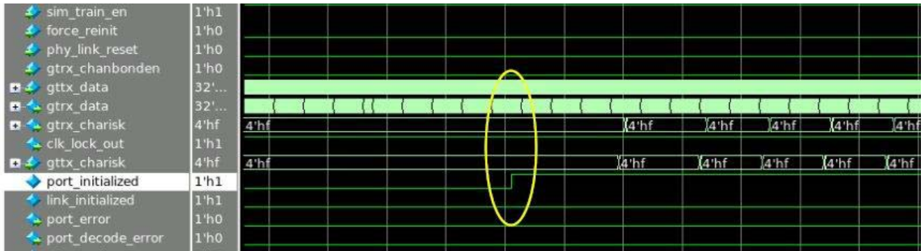
Figure C-3: port_initialized and link_initialized Signals
