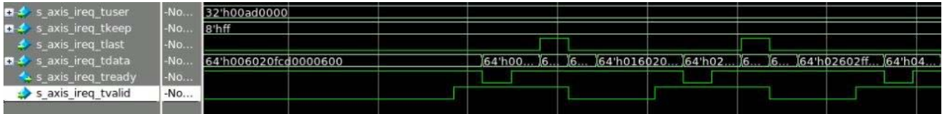
Figure C-7: SWRITE Packet Transmission on IREQ Interface
