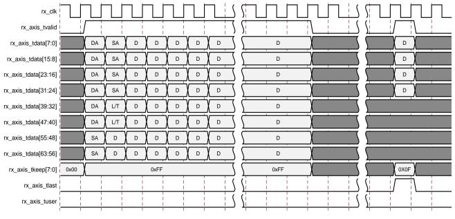
Figure 3-19: Frame Reception with Error
