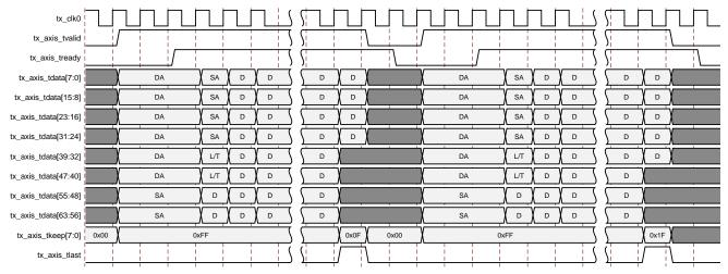
*Figure 3-6:* **Frame Transmission**
