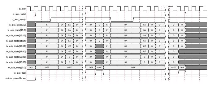
*Figure 3-12:* Transmission of Custom Preamble in the Continuous Case
