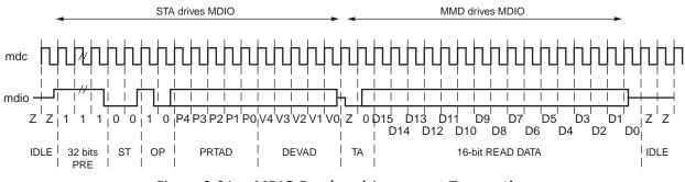
Figure 3-31: MDIO Read-and-Increment Transaction
