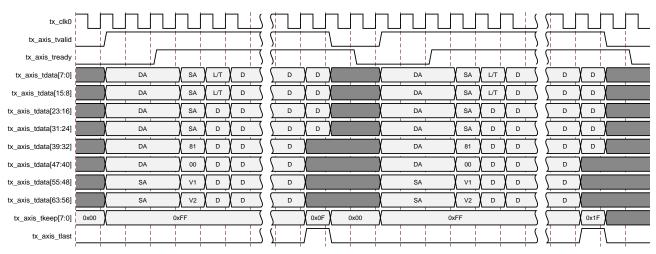
Figure 3-14: VLAN Tagged Frame Transmission
