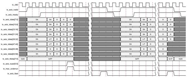
*Figure 3-8:* Frame Transfer Abort with tx\_axis\_tuser asserted
