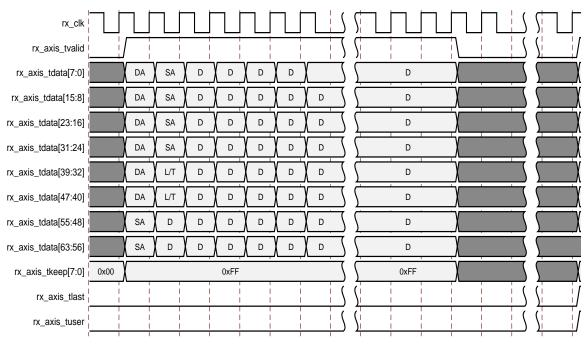
Figure 3-20: Frame Reception with In-Band FCS Passing
