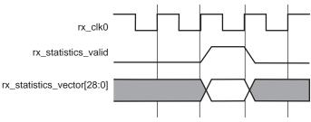
Figure 3-33: Receiver Statistics Output Timing
