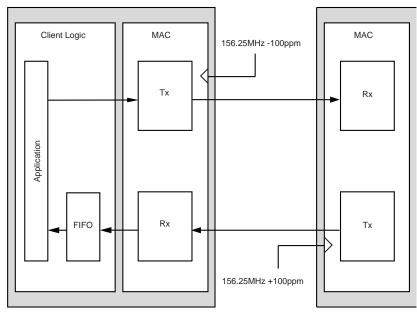
*Figure 3-34:* **The Requirement for Flow Control**
