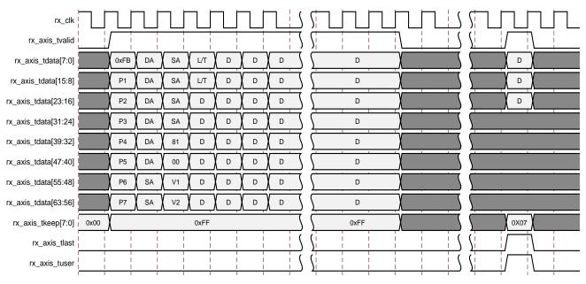
*Figure 3-22:* Frame Reception with VLAN Tagged Frames
