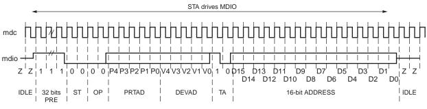
Figure 3-28: MDIO Set Address Transaction
