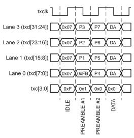
Figure 3-13: XGMII Frame Transmission of Custom Preamble
