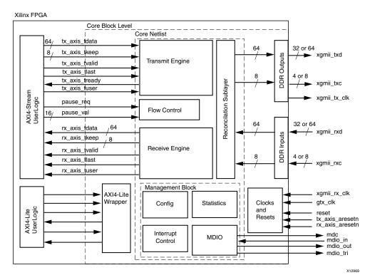
Figure 2-1: Implementation of the 10-Gigabit Ethernet MAC Core
