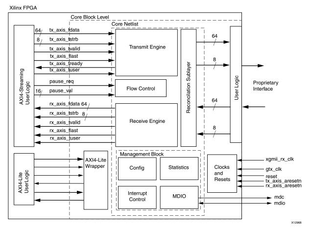
Figure 2-2: Implementation of the Core with User Logic on PHY Interface
