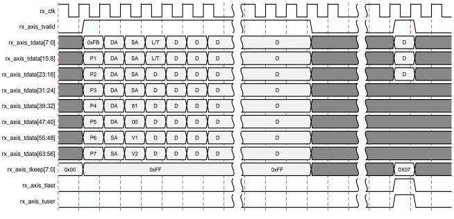
Figure 3-21: Frame Reception with Custom Preamble
