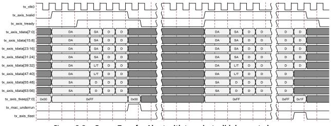
Figure 3-9: Frame Transfer Abort with tx\_axis\_tvalid deasserted
