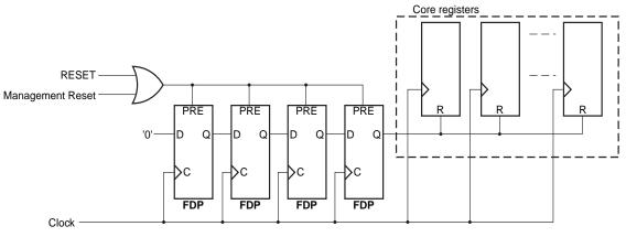
Figure 3-2: Reset Circuit for a Single Clock/Reset Domain
