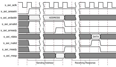
Figure 3-25: Management Register Read Timing
