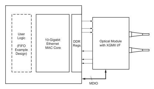
Figure 1-3: 10-Gigabit Ethernet MAC Core Connected to PHY with XGMII Interface
