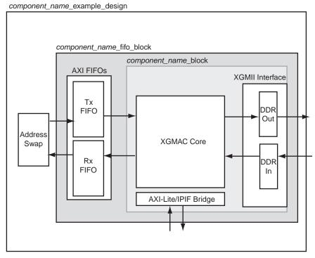
*Figure 7-1:* Example Design and HDL Wrapper for **10-Gigabit Ethernet MAC with XGMII Interface**
