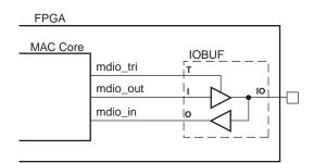
Figure 3-27: Using a SelectIO Interface 3-State Buffer to Drive MDIO
