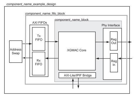
*Figure 7-3:* Example Design and HDL Wrapper for 10-Gigabit Ethernet MAC with 64-bit Interface
