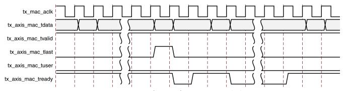
Figure 3-20: Back-to-Back Frame Transmission
