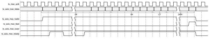
Figure 3-15: Normal Frame Transmission at 1 Gb/s Across User Interface
