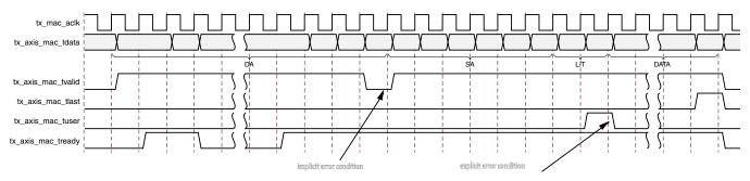
Figure 3-19: Frame Transmission with Underrun
