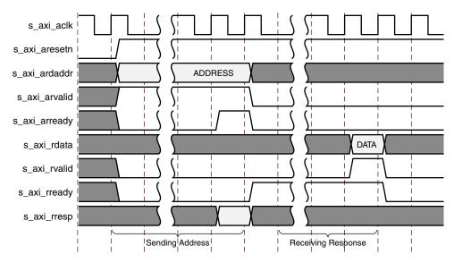
Figure 3-44: Management Register Read Timing
