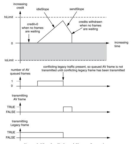
Figure 3-37: Credit-Based Shaper Operation
