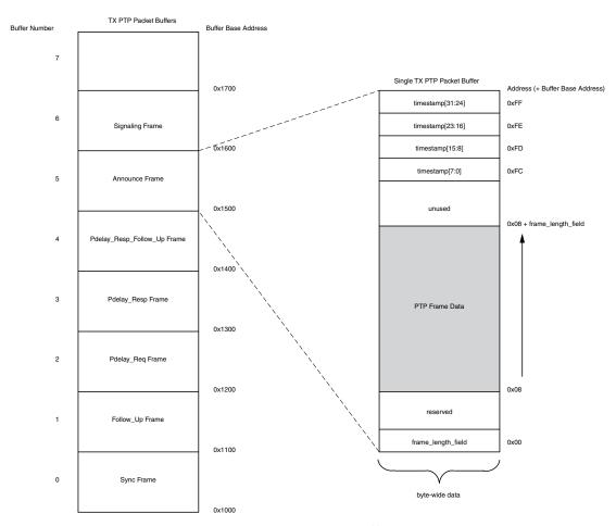
Figure 3-41: TX PTP Packet Buffer Structure
