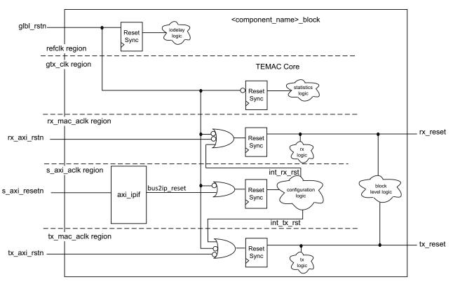
Figure 3-3: Reset Architecture
