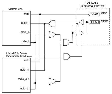
Figure 3-49: Internal and External MDIO Interfaces
