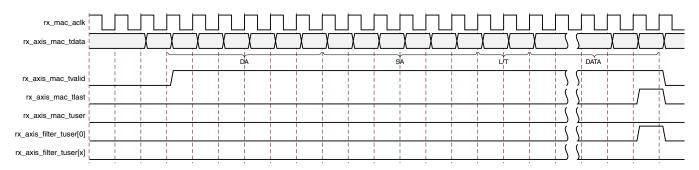
Figure 3-32: Received Frame with No Match on Configurable Frame Filters
