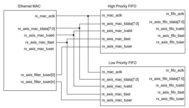
Figure 3-33: Priority FIFO Connections
