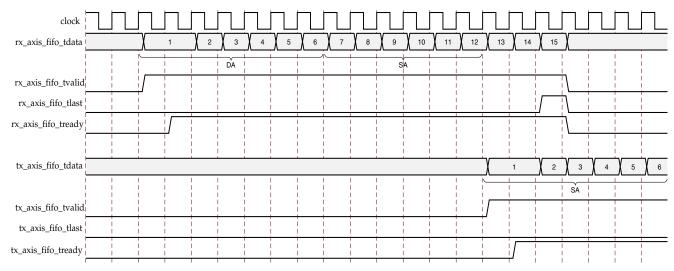
Figure 6-3: Modification of Frame Data by Address Swap Module
