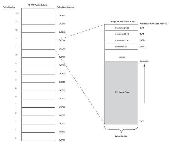
Figure 3-42: RX PTP Packet Buffer
