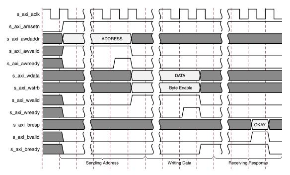
Figure 3-43: Management Register Write Timing
