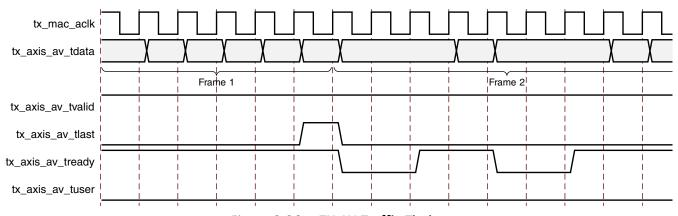
Figure 3-36: TX AV Traffic Timing
