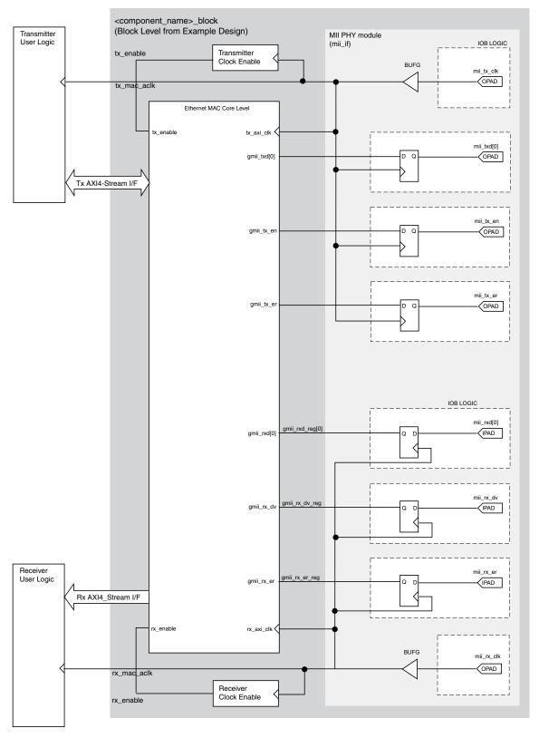
Figure 3-50: MII Transmitter, Receiver and Clock Logic For All Devices
