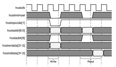
Figure C-3: Host Interface MAC Configuration Read/Write
