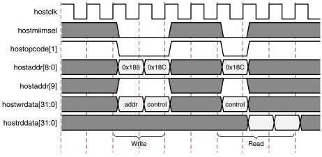
Figure C-4: Address Filter Read/Write
