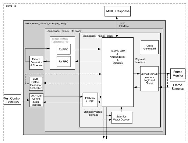
Figure 6-6: Demonstration Test Bench
