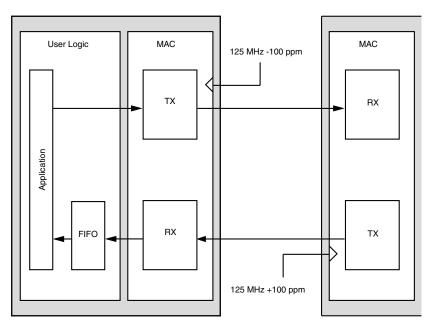
Figure 3-26: Requirement for Flow Control
