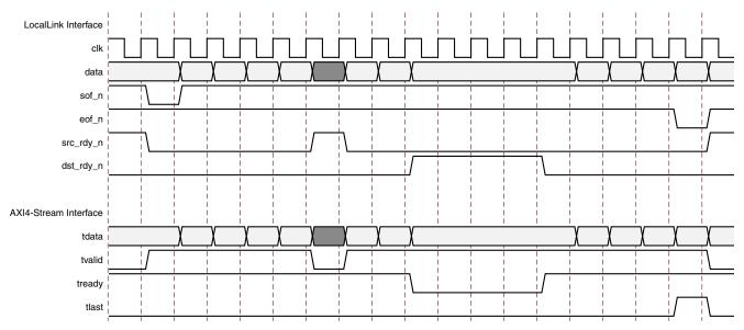
Figure C-11: LocalLink versus AXI4-Stream
