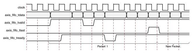
Figure 6-2: Frame Transfer across AXI4-Stream Interface
