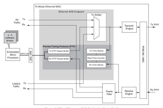
Figure 3-35: Ethernet AVB Endpoint Data Path
