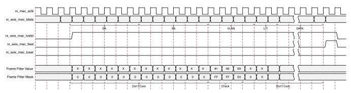
Figure 3-34: Filtering of VLAN Frames with VLAN Priority of 7
