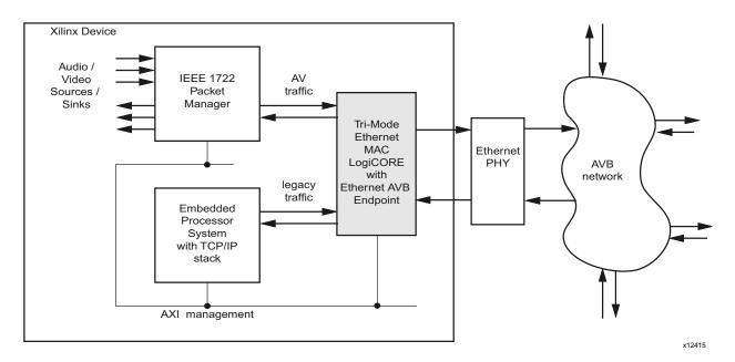
Figure 1-5: Ethernet AVB Endpoint system
