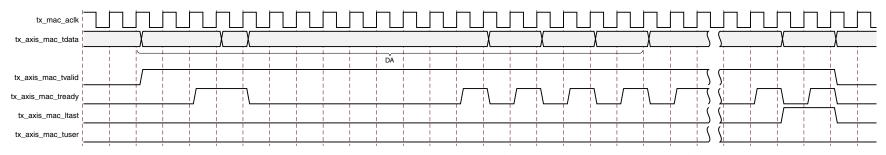
Figure 3-16: Normal Frame Transmission at 100 Mb/s Across User Interface (MII/GMII)
