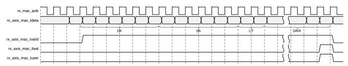
Figure 3-11: Frame Reception with Error
