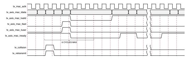
Figure 3-22: Collision Handling – Frame Retransmission Required
