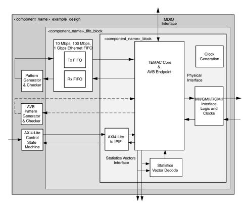
Figure 3-1: Tri-Mode Ethernet MAC Core Example Design
