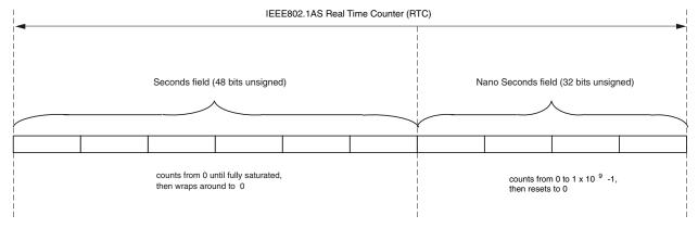
Figure 3-38: Real-Time Clock (RTC)
