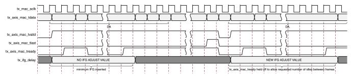
Figure 3-24: Interframe Gap Adjustment
