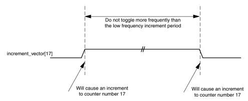
Figure 3-30: Increment Vector Timing Diagram
