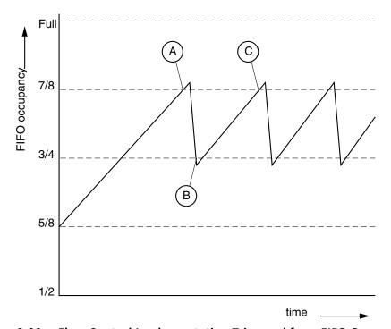
Figure 3-29: Flow Control Implementation Triggered from FIFO Occupancy
