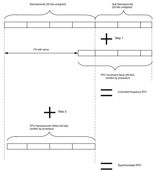
Figure 3-39: Increment of Sub-Nanoseconds and Nanoseconds Field
