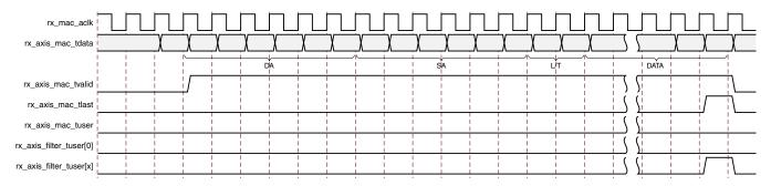
Figure 3-31: Received Frame with a Match on Filter 0
