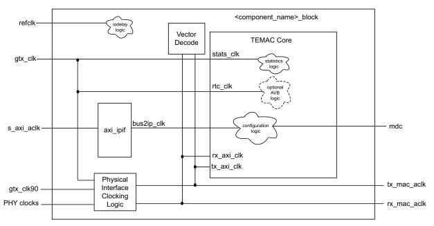
Figure 3-2: Clocking Architecture (Not Including the Physical Interface Clocking)
