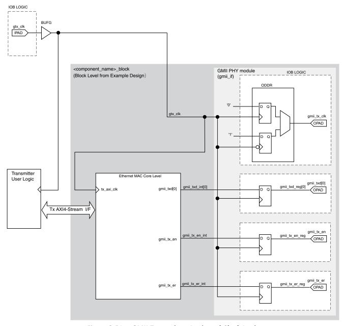
Figure 3-51: GMII Transmitter Logic and Clock Logic
