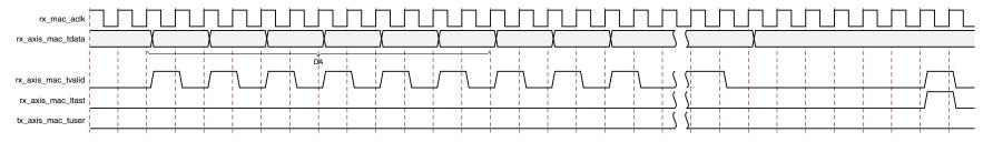
Figure 3-8: Normal Frame Reception at 10/100 Mb/s
