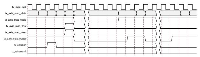
Figure 3-23: Collision Handling - No Frame Retransmission Required
