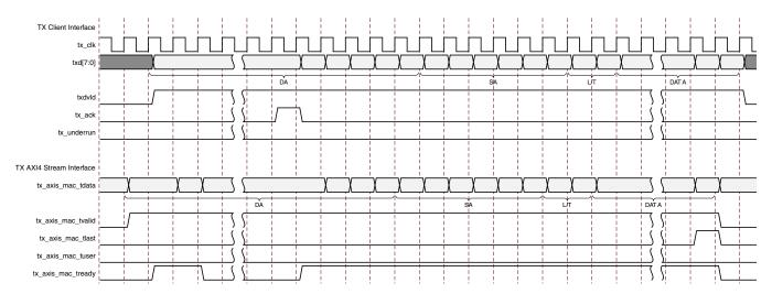
Figure C-9: TX Client Access versus TX AXI4-Stream
