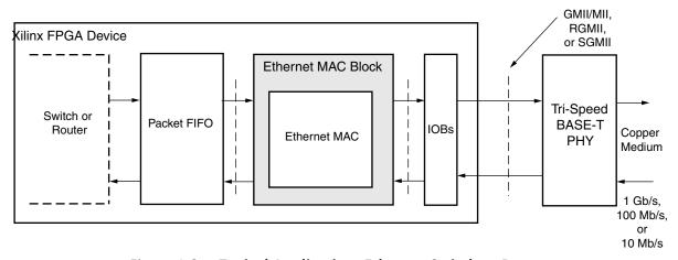
Figure 1-3: Typical Application: Ethernet Switch or Router
