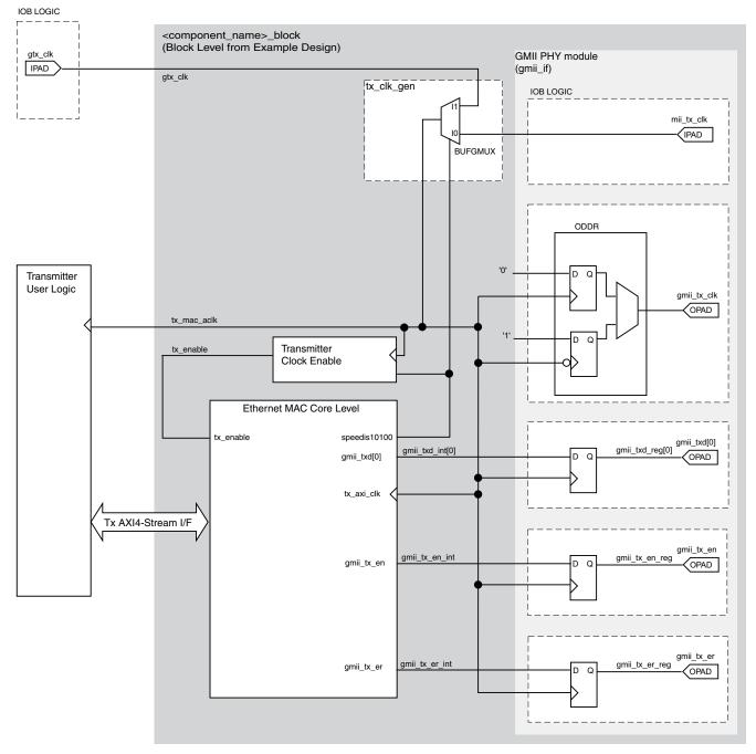
Figure 3-59: GMII Transmitter Logic and Clock Logic
