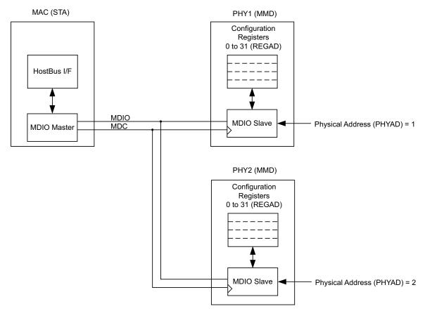
Figure 3-45: A Typical MDIO-Managed System
