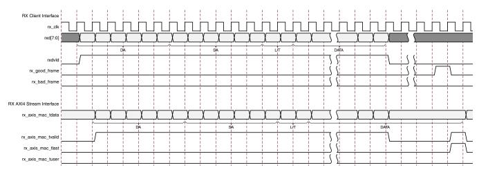
Figure C-10: RX Client Transfer versus RX AXI4-Stream
