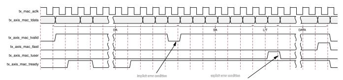
Figure 3-24: Frame Transmission with Underrun
