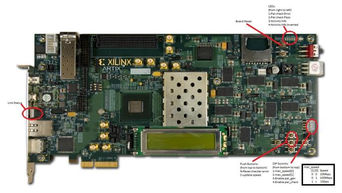
Figure 8-7: AC701 Board Connectivity
