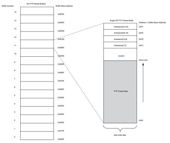
Figure 3-47: RX PTP Packet Buffer
