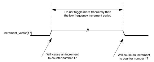
Figure 3-35: Increment Vector Timing Diagram
