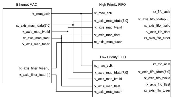
Figure 3-38: Priority FIFO Connections
