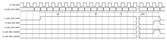
Figure 3-37: Received Frame with No Match on Configurable Frame Filters
