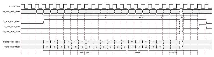
Figure 3-39: Filtering of VLAN Frames with VLAN Priority of 7
