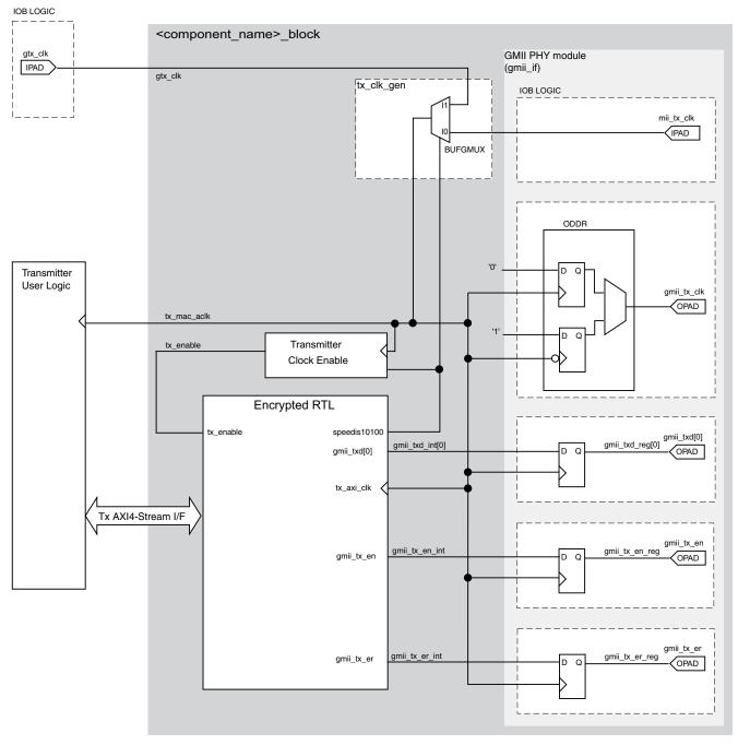
Figure 3-64: Tri-Speed GMII Transmitter Logic and Clock Logic
