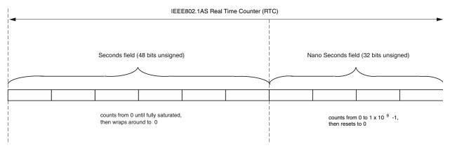
Figure 3-43: Real-Time Clock (RTC)
