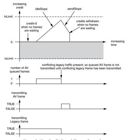
Figure 3-42: Credit-Based Shaper Operation
