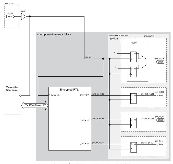
Figure 3-56: 1 Gb/s GMII Transmitter Logic and Clock Logic
