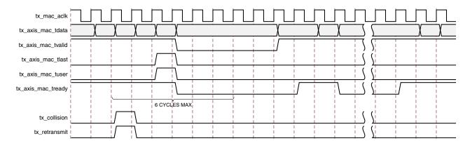
Figure 3-27: Collision Handling - Frame Retransmission Required
