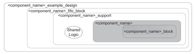
Figure 3-3: Shared Logic Included in Example Design
