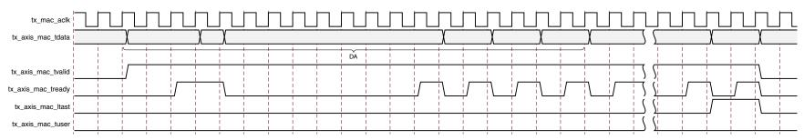
Figure 3-21: Normal Frame Transmission at 100 Mb/s Across User Interface (MII/GMII)
