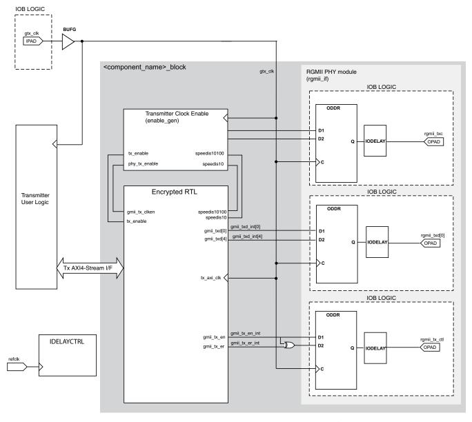
Figure 3-67: Tri-Speed RGMII Transmitter Logic and Clock Logic for 7 Series Devices
