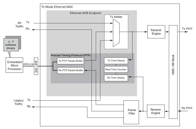
Figure 3-40: Ethernet AVB Endpoint Data Path
