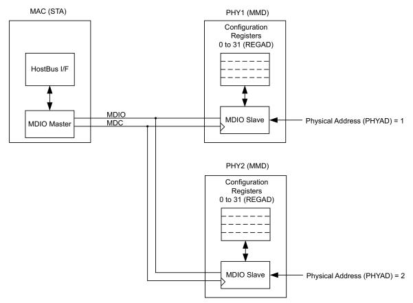
Figure 3-50: A Typical MDIO-Managed System
