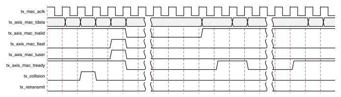
Figure 3-28: Collision Handling - No Frame Retransmission Required
