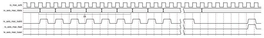
Figure 3-13: Normal Frame Reception at 10/100 Mb/s
