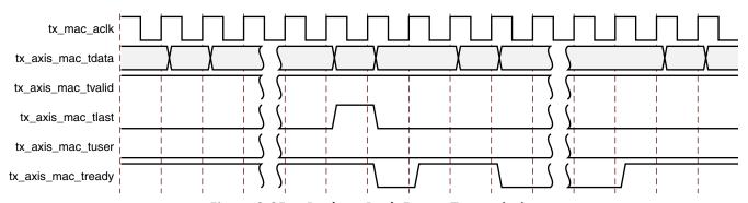
Figure 3-25: Back-to-Back Frame Transmission
