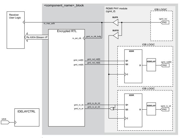
Figure 3-61: 1 Gb/s RGMII Receiver Logic and Clock Logic for 7 Series Devices
