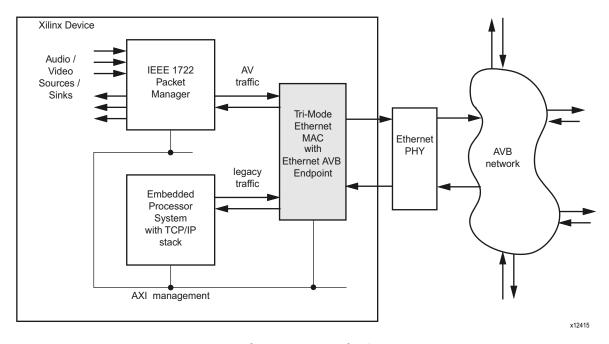
Figure 1-5: Ethernet AVB Endpoint System
