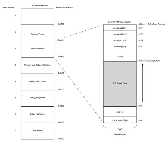
Figure 3-46: TX PTP Packet Buffer Structure
