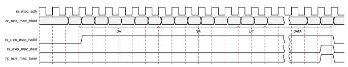
Figure 3-16: Frame Reception with Error
