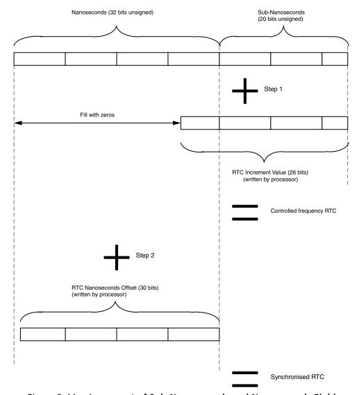
Figure 3-44: Increment of Sub-Nanoseconds and Nanoseconds Field
