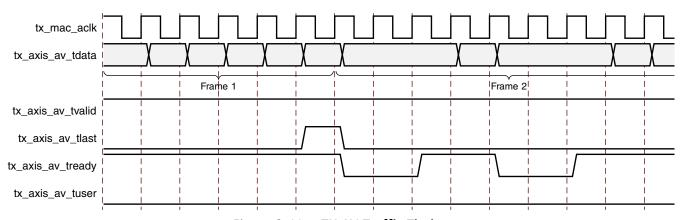
Figure 3-41: TX AV Traffic Timing
