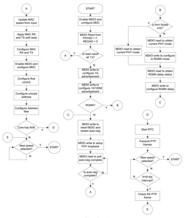
Figure 8-5: State Machine Flow Diagram
