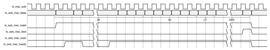
Figure 3-20: Normal Frame Transmission at 1 Gb/s Across User Interface
