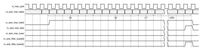
Figure 3-36: Received Frame with a Match on Filter 0
