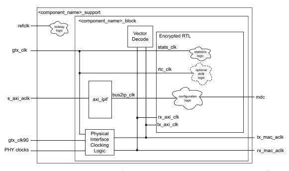
Figure 3-7: Clocking Architecture (Not Including the Physical Interface Clocking)
