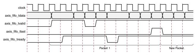
Figure 8-2: Frame Transfer across AXI4-Stream Interface
