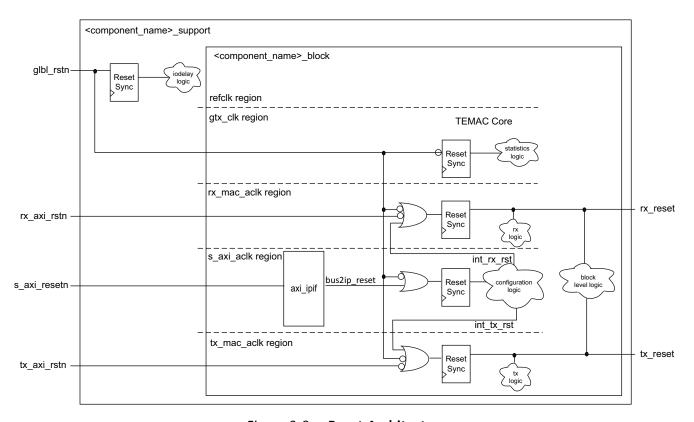
Figure 3-8: Reset Architecture
