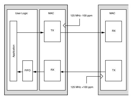
Figure 3-31: Requirement for Flow Control
