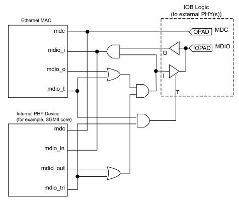
Figure 3-54: Internal and External MDIO Interfaces
