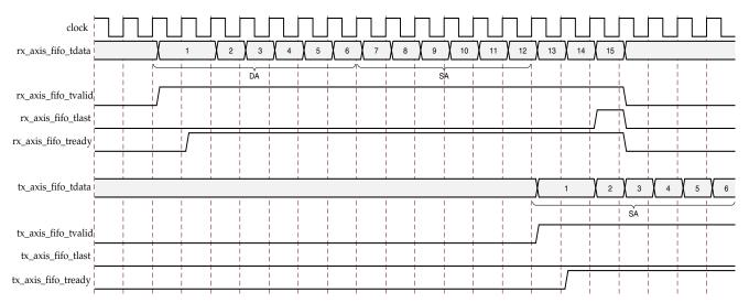
Figure 8-3: Modification of Frame Data by Address Swap Module
