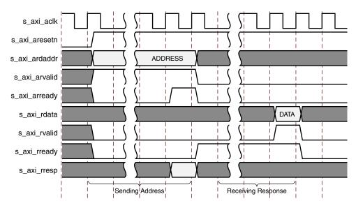
Figure 3-49: Management Register Read Timing
