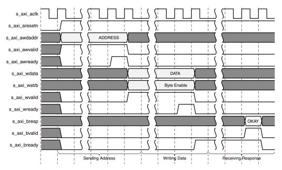
Figure 3-48: Management Register Write Timing
