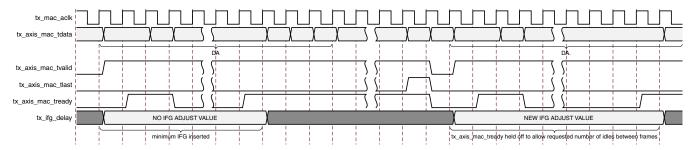
Figure 3-29: Interframe Gap Adjustment
