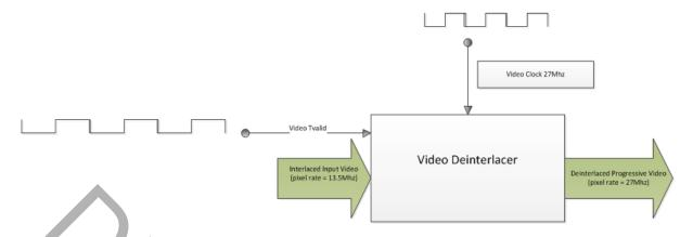
Figure 3-8: Input to Output Video Clock Ratio for SD
