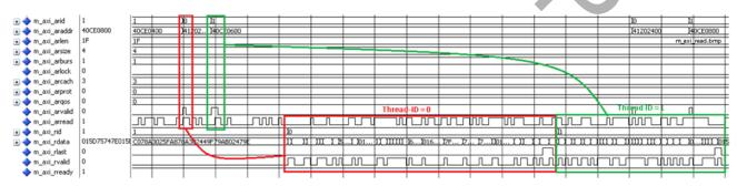
Figure 3-7: Read Stream Burst
