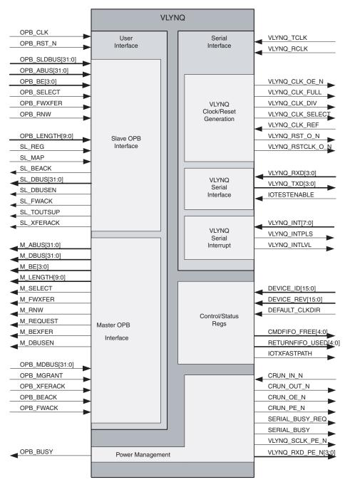
Figure 6: VLYNQ Core Interfaces
