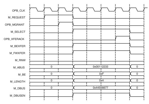
Figure 7: VLYNQ Core Mastering OPB Bus: Single Write
