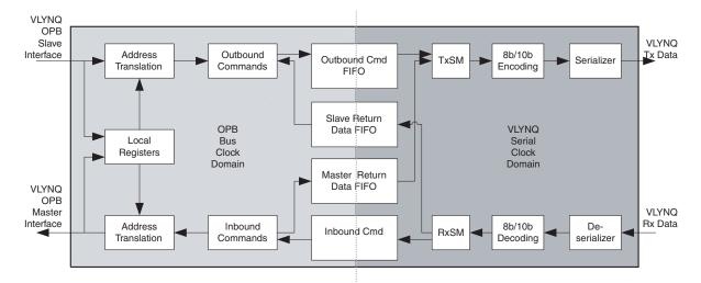
Figure 2: VLYNQ Core Block Diagram
