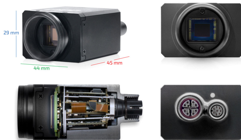
Figure 7: Triton Edge Camera with InFO Packaging
